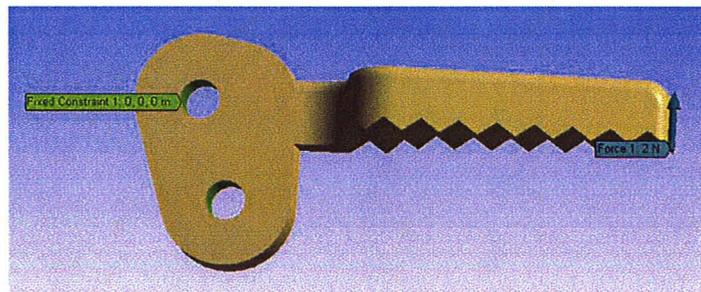
Figure B.37 Loading used for stress analysis of top gripper jaw.
