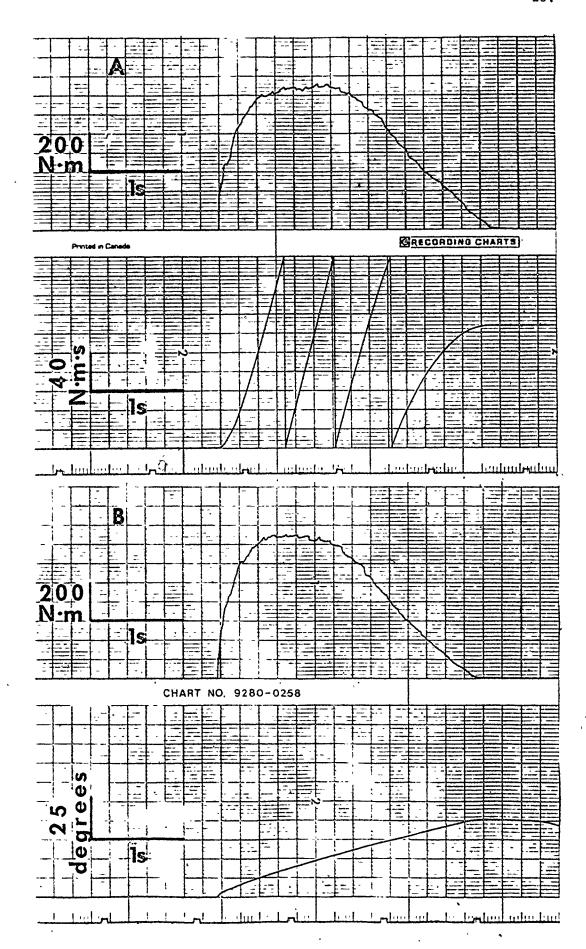
integration of torque and time and permitted the measurement of impulse in newton-metre-seconds (N.m.s), and average torque, measured as the impulse divided by the time of the contraction. Values for peak torque, average torque and impulse can be converted to peak power (W, watts), average power (W) and work (J, joules), respectively, by multiplying by the lever arm velocity (in rad/s, rad = radians, 1 radian = 57.3°/s.
