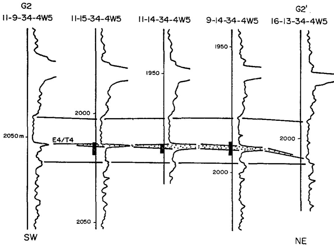
Figure 4.7. Well log cross sections G3 and G4 from Garrington, located in Figure 4.1. The Burnstick Member is shown with dots and is bracketed by the lower and upper markers.
