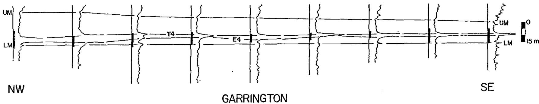
Figure 4.20. Cross section YY' from Crossfield. This cross section is oriented parallel to the strike of Crossfield. Note the decrease in grain size from the northern part of the cross section into the southern part of the cross section.
