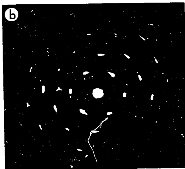
Fig. 7.4 InP single crystal photochemically thinned. a) Bright field micrograph showing structure of a surface prepared by polishing with 1 \mu\text{m} sized particles. b) Corresponding selected area electron diffraction pattern showing spot splitting indicative of a high degree of crystal damage.
