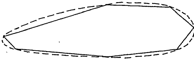
Fig. 3.3.2. Approximating the pocket with straight-line segments in order to be able to use the "POCKET" routine.
