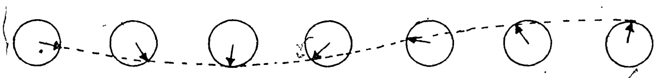
Fig. 2.1(c) Wavelike form of the precession of spins when viewed from above.
