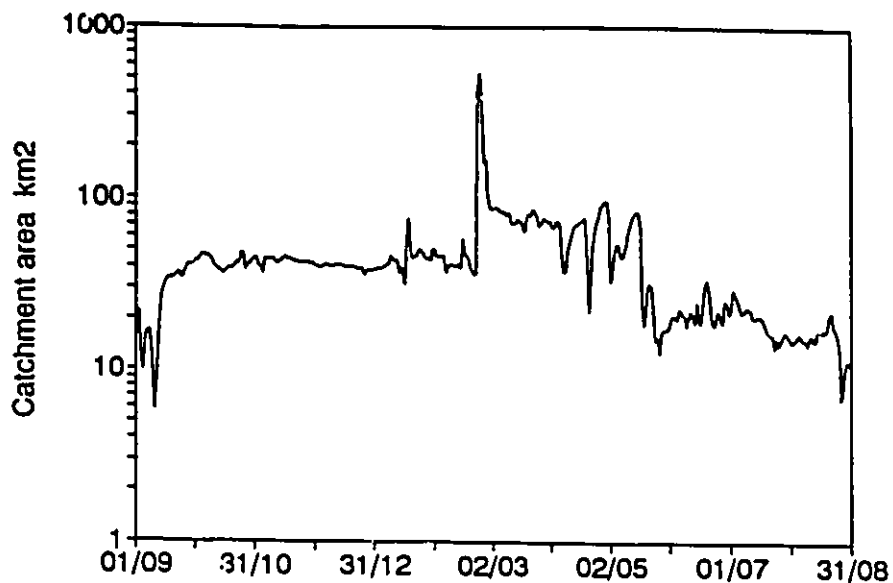
Figure 9.15 Calculated catchment area for Crowsnest Spring, assuming identical specific discharge to Ptolemy Spring
