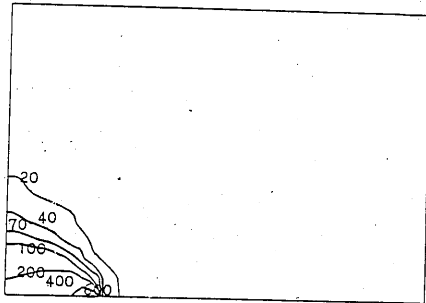
FIG. 6.11 EVOLUTION OF TEMPERATURES (°C) AT t=23.28 sec.
