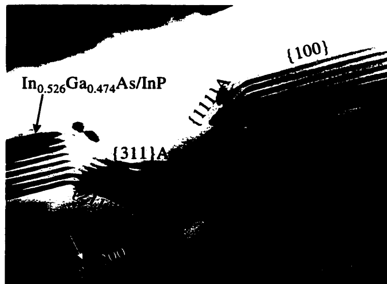
Fig. 6.4 DF TEM image of sample 489(211)A (layers in 0.103% compression) with \vec{g} = 022 .
