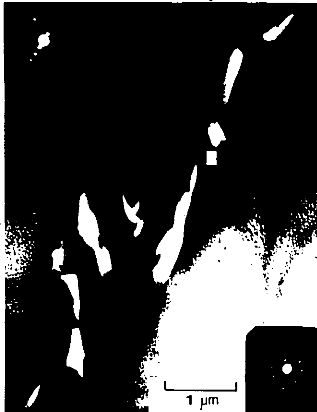
Fig. 48 Grain boundary migration preceding the onset of discontinuous precipitation. 478K, 300 s. STEM micrograph 20K ×.
