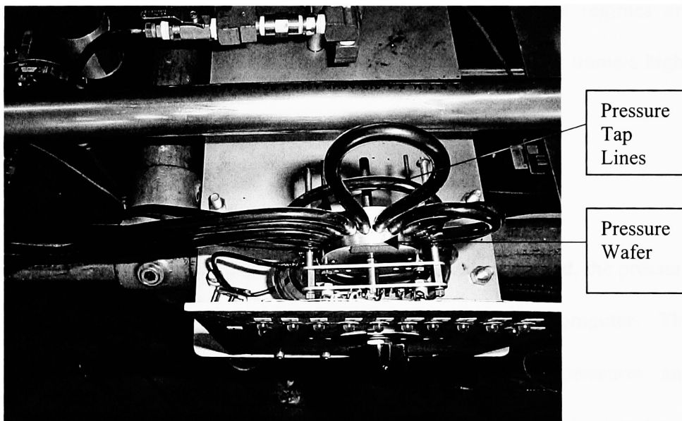
Figure 4.8: Scanivalve Pressure Wafer (From Above)
