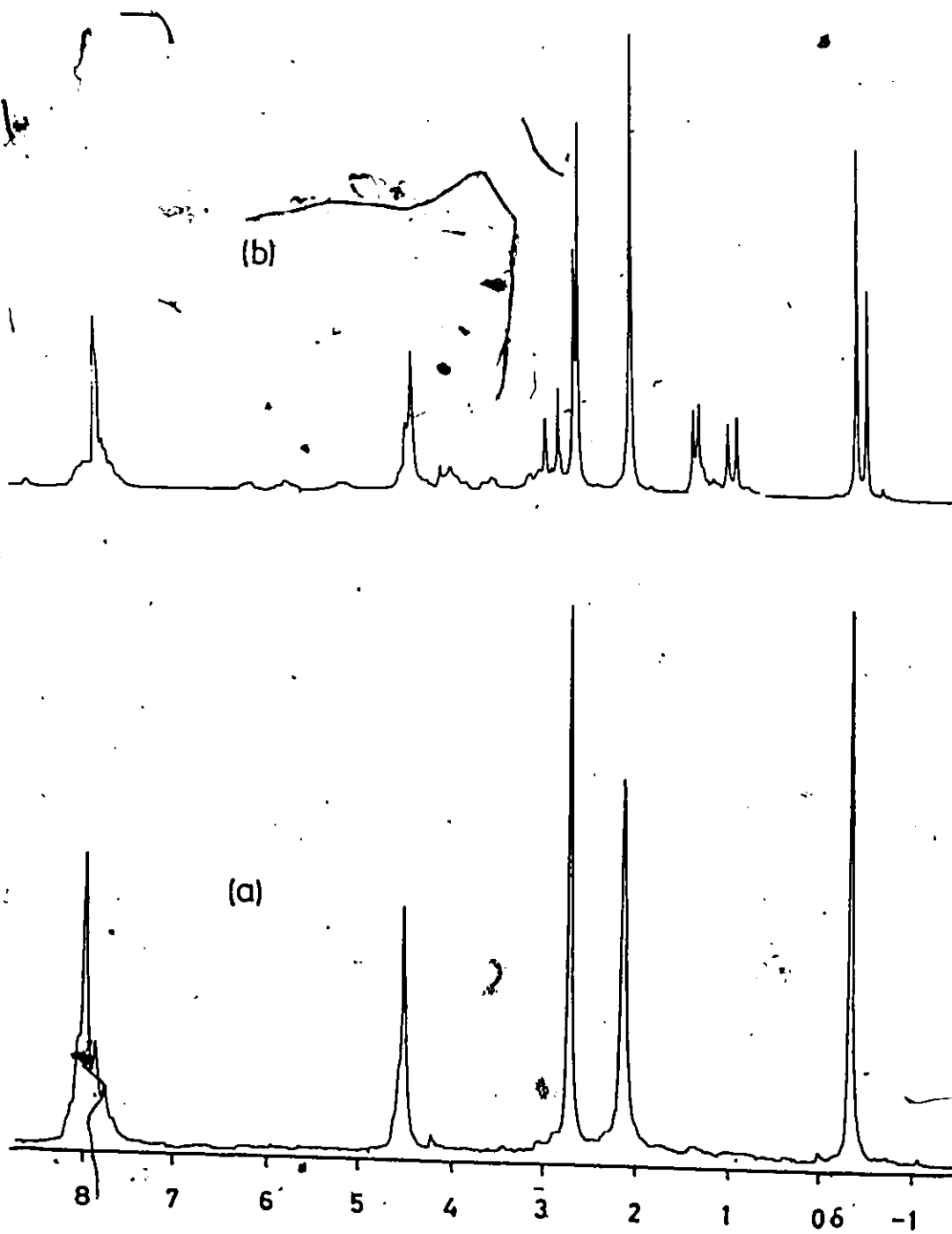
Figure 15 ^1\text{H} NMR spectrum of a solution of the alcohol 157 in \text{FSO}_3\text{H}/\text{SO}_2\text{ClF} (a) at -100^\circ\text{C} and (b) at -70^\circ\text{C} for 1 hour.
