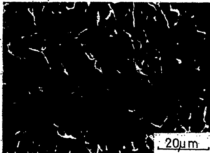
Figure 5.19: SEM-micrograph showing fracture surface of delamination failure propagating along ferrite grain boundaries.
