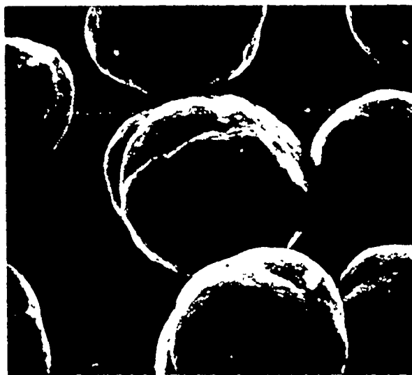
Figure 69. SEM Micrograph of As-received Nickel Powder.
