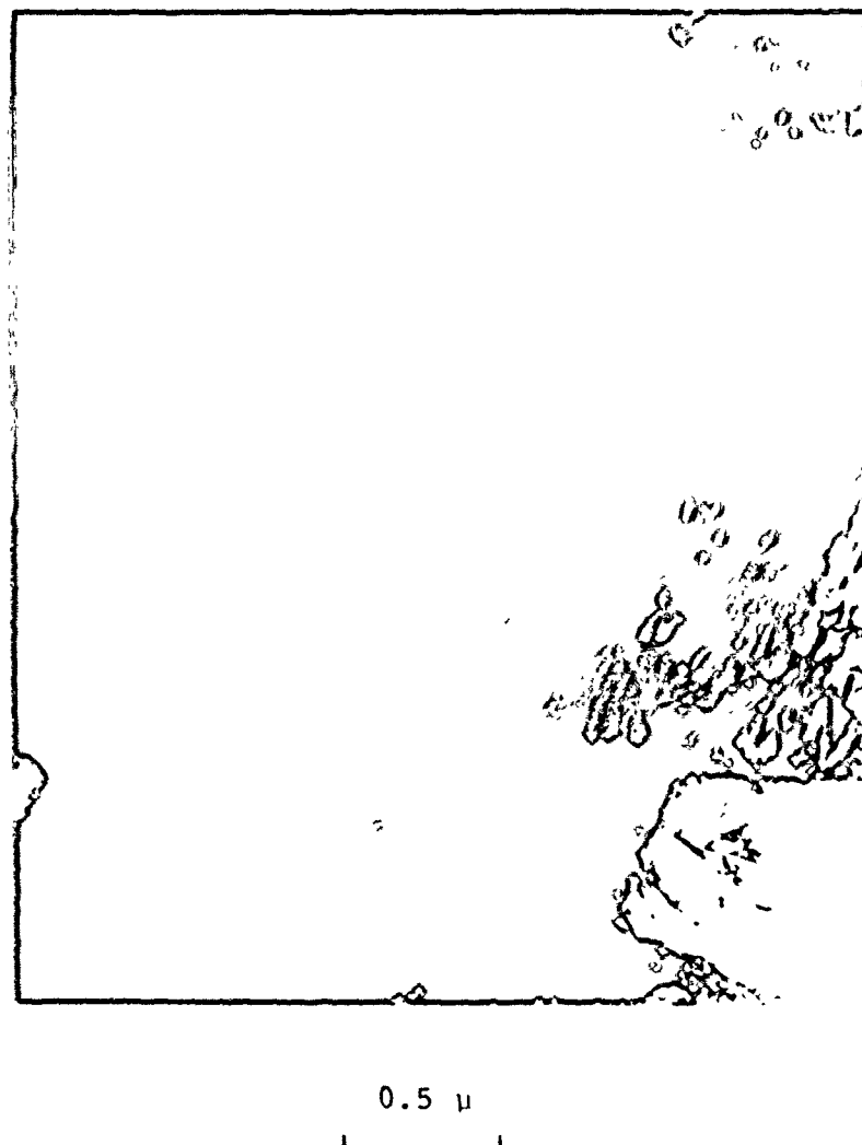
Fig. 20: Structure of a cell wall at fatigue saturation in decarburized iron
