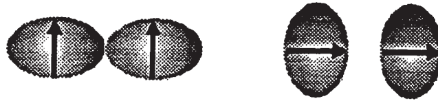
Fig. 2.13 - Spin-orbit coupling deforms the electronic distribution of the atom and ties it to the spin orientation. Adjacent atoms experience an anisotropic exchange interaction due to the difference in electronic overlap when the spins rotate.
