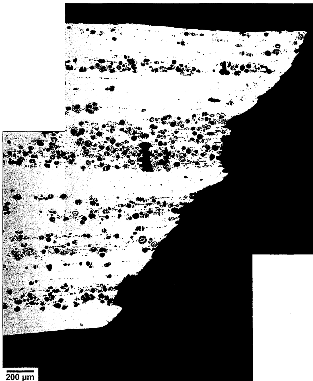
Figure 3.16. Optical micrograph of a fracture surface cross-section in a sample with an average 7.8% volume fraction. Note the linkage of damage between cracked particles visible in the high volume fraction region.
