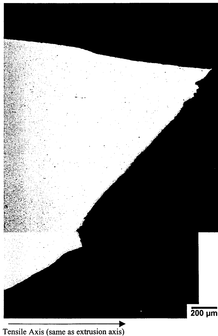
Figure 3.14. Optical micrograph of a fracture surface section for a composite possessing a measured 0% volume fraction of \text{Al}_2\text{O}_3 .
