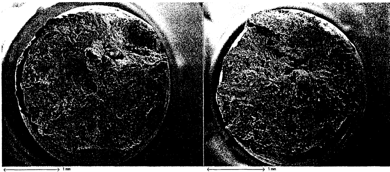
Figure 3.10. Matching fracture surfaces of the 4% volume fraction composite. A sample manufactured from the same composite material is later used in the tomography work. The area of the fracture surface was calculated directly from the image on the left.
