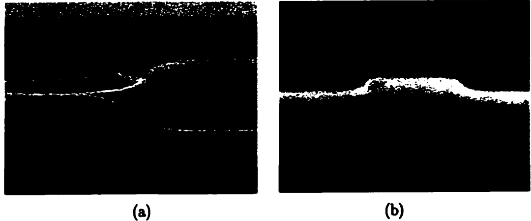
Figure 6.4: LOCOS optical waveguides in SiGe. (a) The structure after several hours in an oxidizing furnace, showing the masking layer and the field oxide. (b) The structure after removal of the \text{SiO}_2/\text{Si}_3\text{N}_4 mask and the thermal oxide.
