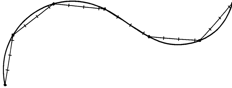
FIGURE 2-6 Linear interpolation of a general spatial curve. The dots denote points p_i on the tool-path. The points are linearly interpolated with the hash marks spaced apart a distance f\Delta t or less. The cutter travels from left to right.
