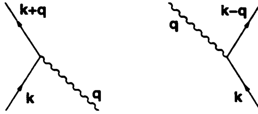
Figure 2.1: The adsorption and emission of phonons is depicted by their Feynmann diagrams. On the left is depicted the adsorption of a phonon of momentum q (wavy line) by an electron of initial momentum k and final momentum k + q . On the right is the inverse process – an electron of initial momentum k emits a phonon of momentum q and the electron has a final momentum k - q .
