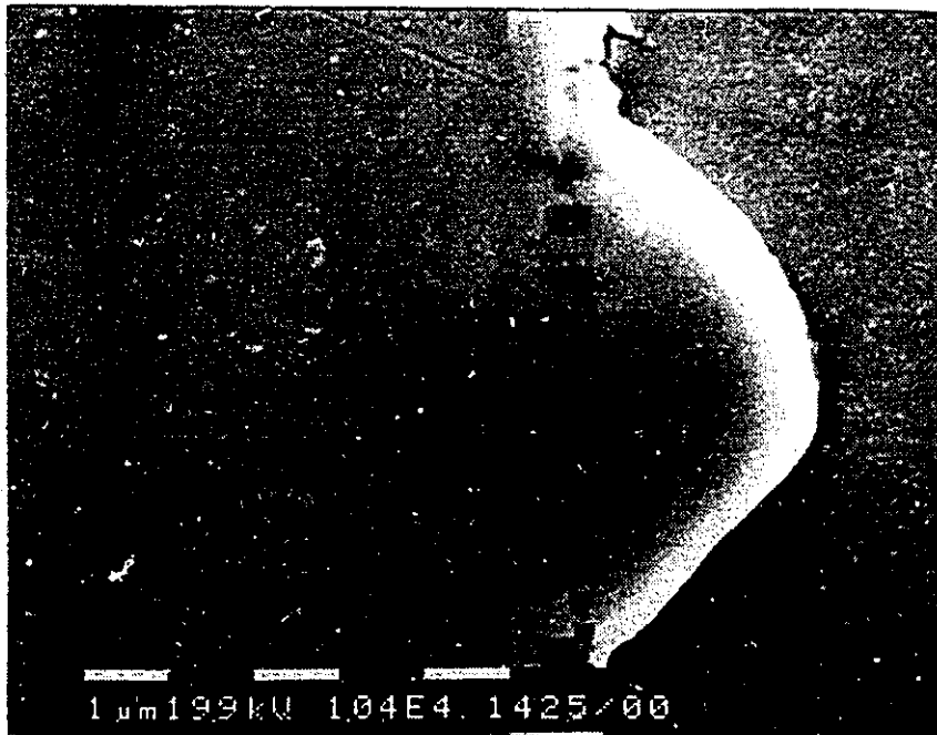
Figure 4.1.10: Cross sections of a 0.5 w/o Ti alloy: nitrided 96 hours at 1020°C in 1 atmosphere nitrogen gas. The large dark particle in the centre of Fig 4.1.10a is an artifact; the precipitation front extends to the arrow b) higher magnification image under 'Ni Cap'
