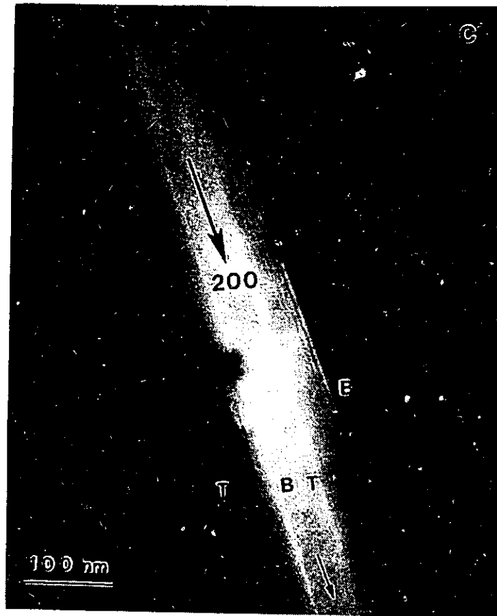
Figure 4.2.10: Weak Beam Dark Field Images of interfacial structure a) g_{\bar{1}\bar{1}}^{\text{Ni}} , w = +1.9 b) g_{\bar{1}\bar{1}}^{\text{Ni}} , w = +1.9 and c) g_{200}^{\text{TiN}} , w = +2.7
