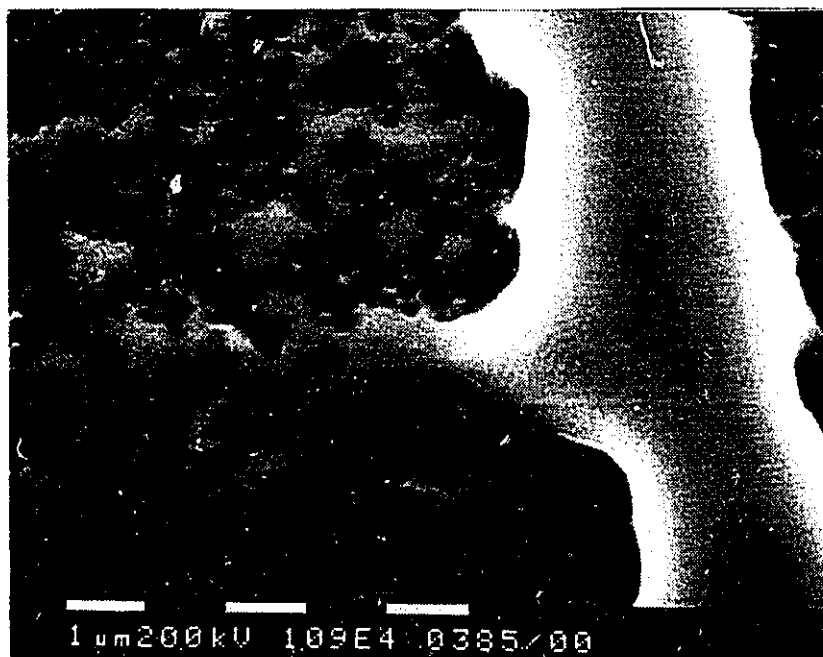
Figure 4.1.6: Surface micrograph of a 0.5 w/o Ti nitrided 96 hours, at 1020°C in 1 atmosphere nitrogen gas a) low magnification b) high magnification
