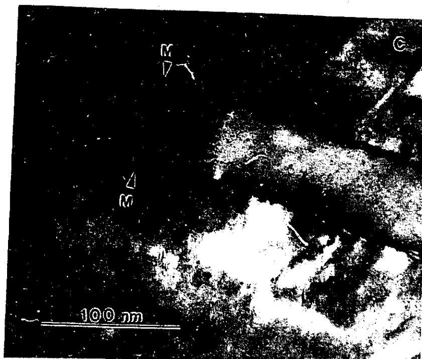
Figure 4.2.21: Example of a particle with a Type V OR a) bright field [110]\text{TiN}||[211]\text{Ni} b) diffraction pattern and c) higher magnification of the interface showing Moiré fringes.
