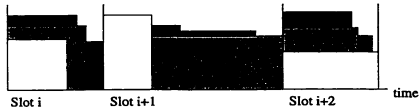
Figure 6.2: SDMA/TDMA frame structure with variable packet size.
