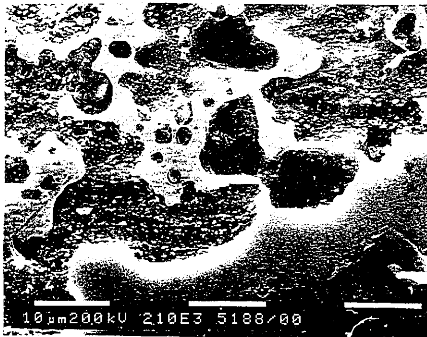
Fig. 5.22. SEM micrograph of a beryllium surface annealed at 773 K for 2 hours before being heated up to 1173 K. The sample was implanted with 2.5 \times 10^{20} 30 keV He/m 2 at room temperature.
