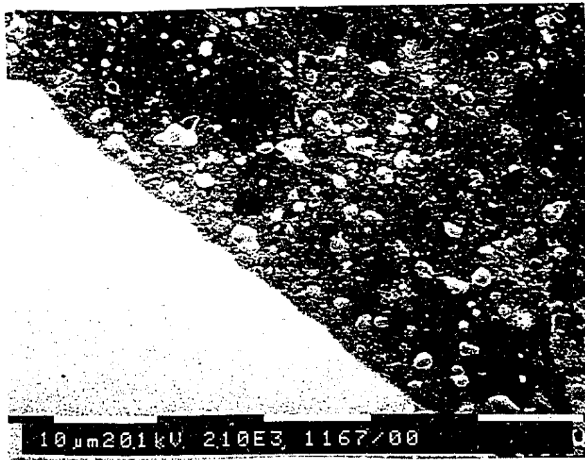
Fig. 5.20. SEM micrograph of a beryllium surface annealed at 573 K for 2 hours before being heated up to 1173 K. The sample was implanted with 2.5 \times 10^{20} 30 keV He/m 2 at room temperature.
