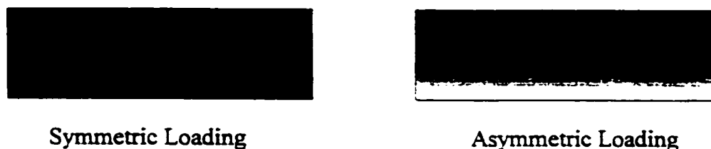
Figure 5.3. Schematic of the gradient gel in an asymmetric pore-filled membrane as compared to a symmetric fill.
