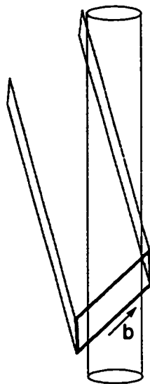
Figure 5.15 Double cross-slip of shear loops around a fibre resulting in a prismatic loop left around the fibre and a prismatic loop in the matrix. Large loops must be produced if cross slip occurs on a system close to the fibre axis. Original shear loop is drawn in black while the two prismatic loops are drawn in gray.
