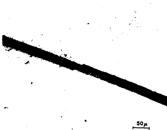
Figure 2.25 Markings on an Fe whisker after the onset of plastic deformation. The localization of strain into slip bands at specific points along the length of the fibre reduces the overall ductility (Brenner, 1958).
