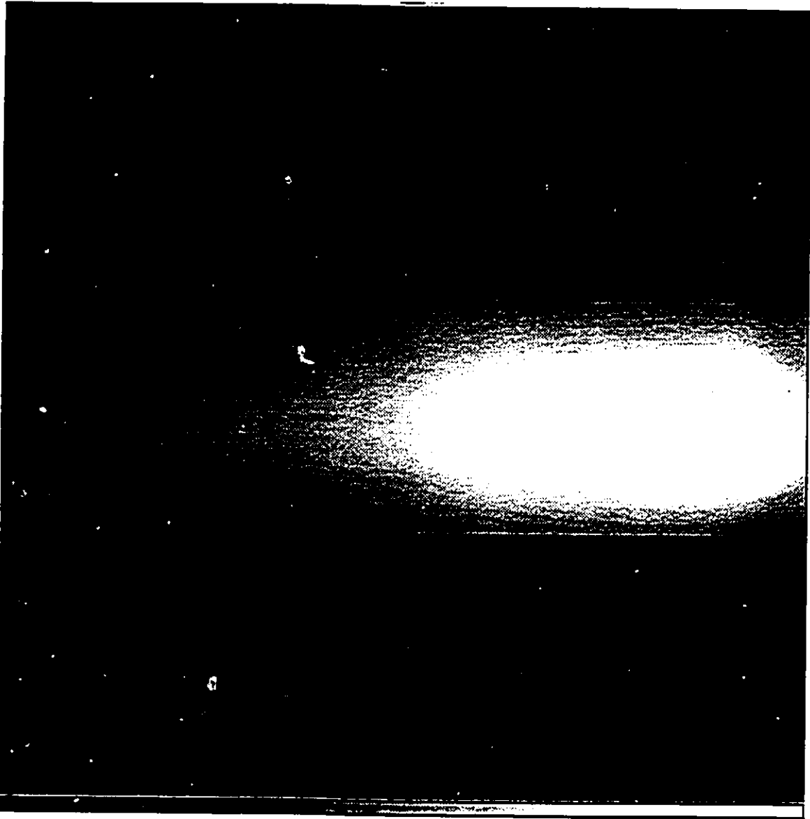
Figure 4.1: An image of the average milk flat, MILK.IMH, obtained by scaling and combining the individual milk flats obtained on the first night of observing. Milk flats are highly defocused spectra of the dome white spot obtained by placing a piece of diffusive opal glass in front of the optical fibers in the spectrograph.
