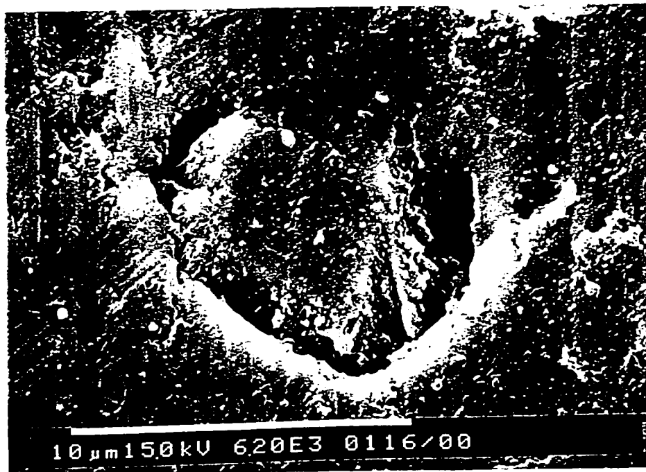
Figure 5.2.4b: SEM images of the chip showing voids formed around SiC particles ( v = 894 m/min., f = 0.35 mm/rev., d = 2.0 mm., \alpha = 0^\circ , r = 1.6 mm)
