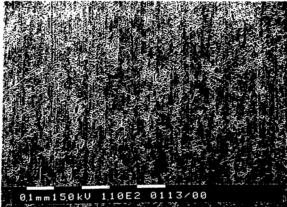
Figure 5.2.4a: SEM images of the chip showing typical topography ( v = 894 m/min., f = 0.35 mm/rev., d = 2.0 mm., \alpha = 0^\circ , r = 1.6 mm)
