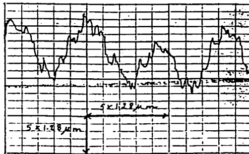
Figure 5.2.17b: Surface roughness profiles of surfaces machined with a chip breaker clamped on top of the PCD insert ( v = 894 m/min, f = 0.35 mm/rev., d = 1.5 mm, r = 1.6 mm, \alpha = 0^\circ ).
