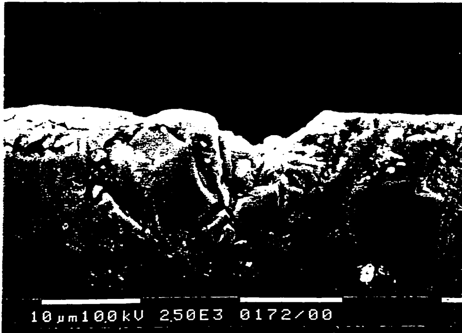
Figure 5.2.4c: SEM images of the chip showing pulled out SiC particles ( v = 894 m/min., f = 0.35 mm/rev., d = 2.0 mm, \alpha = 0^\circ , r = 1.6 mm)
