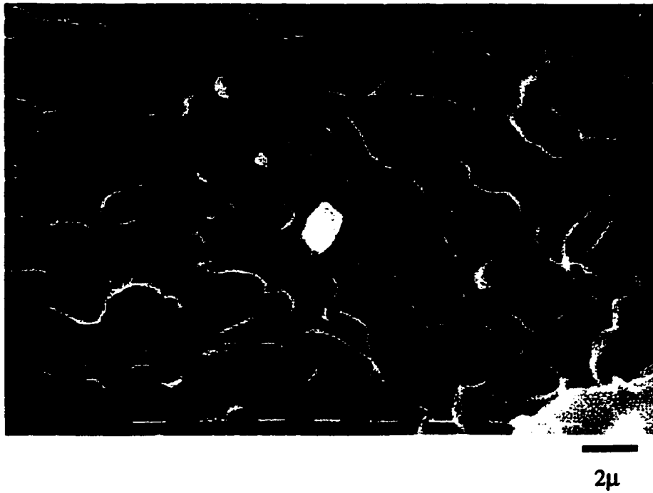
Figure 4.32: SEM microphotograph of fractured surface of rotomolded polypropylene
