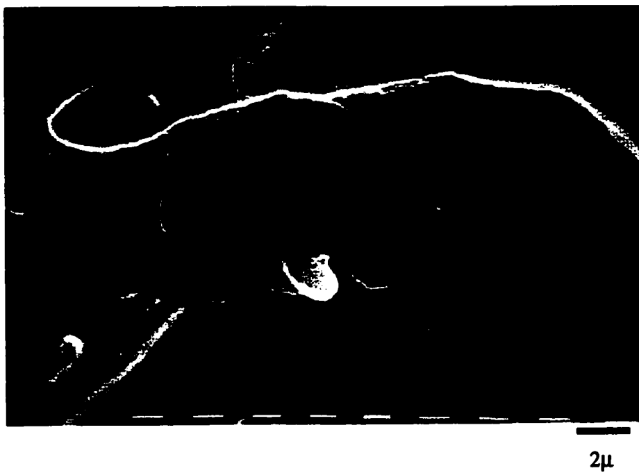
Figure 4.28: SEM microphotograph of fractured surface of rotomolded EBA
