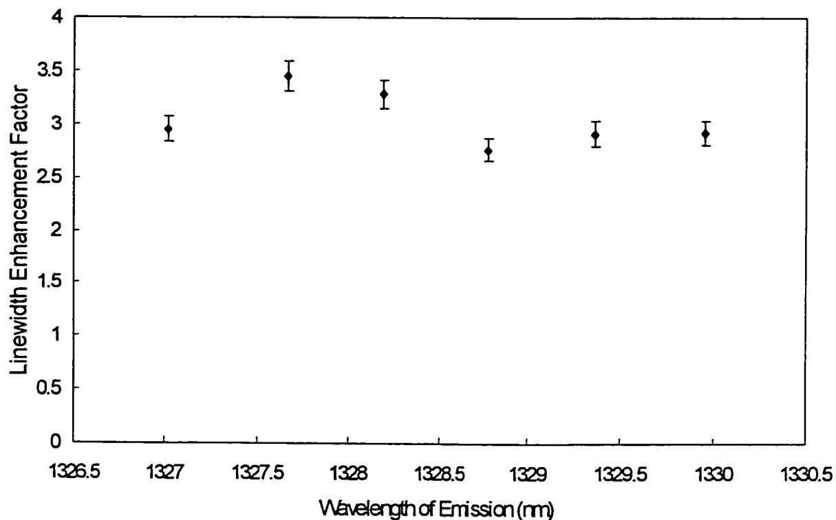
Figure 21: Linewidth Enhancement Factors of S1-590. Mode 5 is near the gain peak of the laser.
