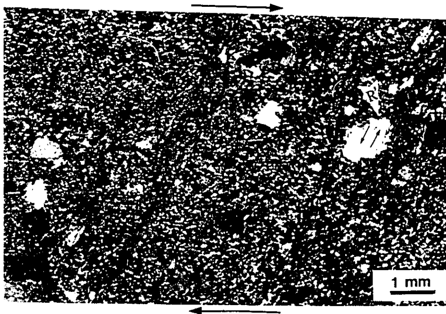
Figure 4.24, Photomicrograph of mylonitic fabrics with displaced broken feldspar. Microfractures within the feldspar correspond to the antithetic Riedel shear (R') and has opposite sense of shear to the main shear zone.
