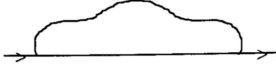
Figure 2.4 Lowest order contribution the electronic self-energy from the electron-phonon interaction. The wavy line is the phonon propagator and the solid line is the electron propagator.
