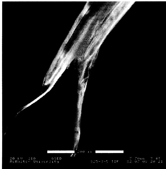
Figure 2.10 SEM micrograph of a broken specimen of nascent PE microfiber produced in Run 2 during tensile test.
