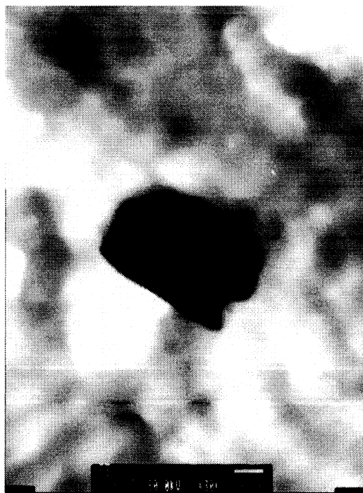
Figure 2.10 TEM photograph of the polymer produced in Run 21 with MSF-Ni catalyst (scale bar: 0.2 \mu\text{m} ), showing a silica fragment (dark area).
