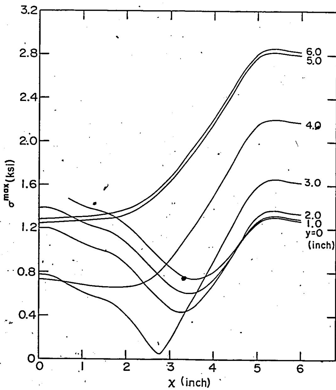
support, the total tensile stress acting upon each bar is  $\sim 2.1$  ksi, for 10-atm pressure in the chamber. This stress is smaller than the bending stress induced in the end plate.
