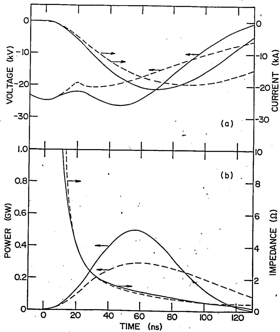
the second peak in the discharge voltages (Figs. 3-33(a), 3-34(a) and 3-35(a)) is due to the continuing transfer of energy from the storage capacitor. For low-pressure discharges, however, one may expect an abrupt drop in the discharge voltage corresponding to a rapid rise in the main discharge current.
