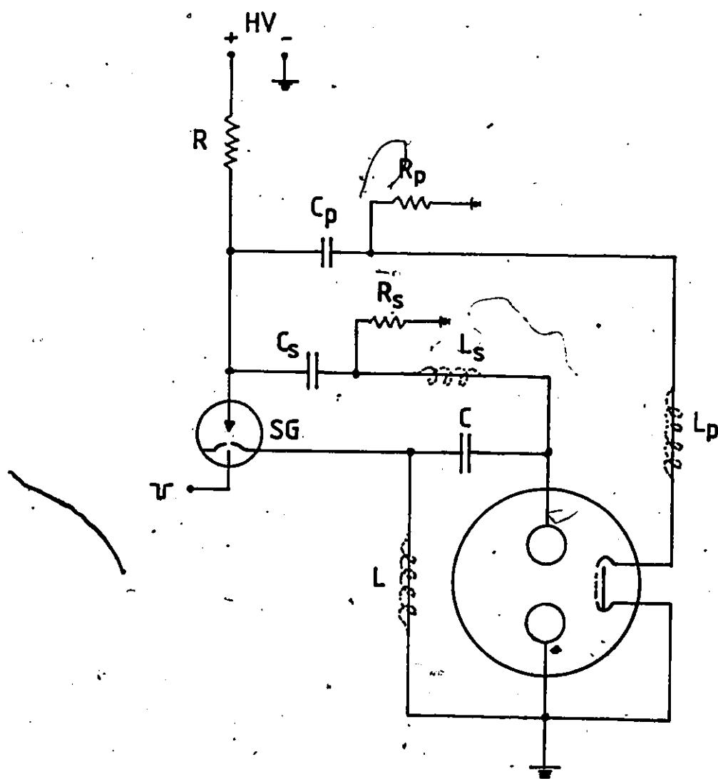
pressure, the electrode separation and the applied voltage. It should be noted that the ceramic capacitors are not located inside the discharge chamber and close to the electrodes, as done in Ref.[96]. Instead, they are mounted externally, and use the supporting structure to increase the circuital inductance L in order to broaden the discharge current pulse.
