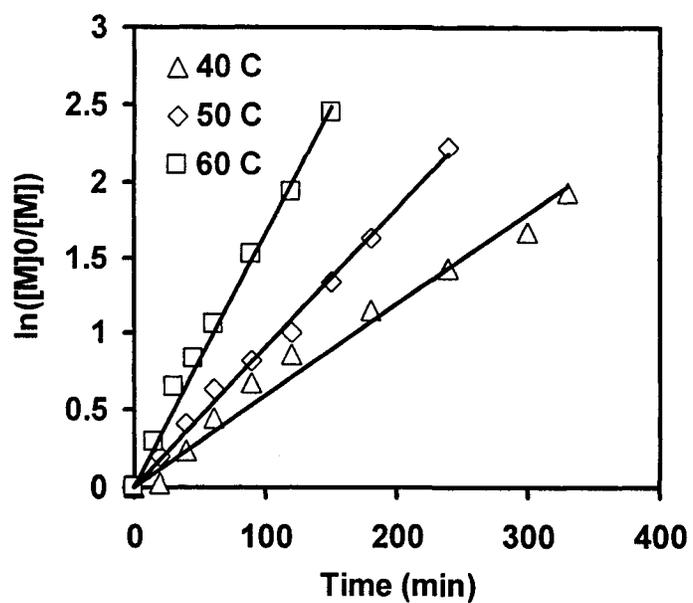
**Figure 3.3.**  $\ln([M]_0/[M])$  of THF solution polymerization of DMAEMA vs time at 40, 50 and 60 °C with  $[DMAEMA]_0 = 2.96$  (mol/L) and  $[ABIB]_0 = [CuBr]_0 = [PMDETA]_0 = 0.0296$  (mol/L)
