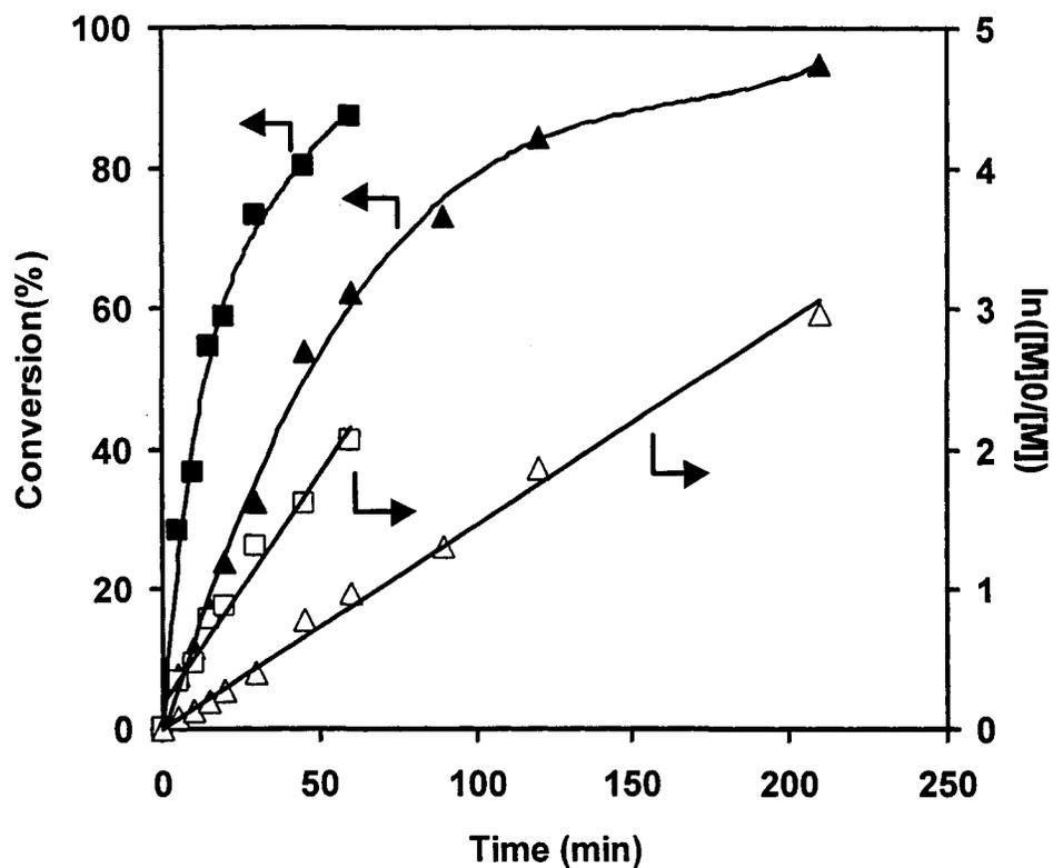
**Figure A1.** The aqueous ATRP of DMAEMA catalyzed by CuBr-Bpy at 20 and 30 °C.  $[\text{DMAEMA}]_0/[\text{MBP}]_0/[\text{CuBr}]_0/[\text{Bpy}]_0 = 100:1:1:2$  in mole, DMAEMA/D<sub>2</sub>O = 1:1 (w/w).
