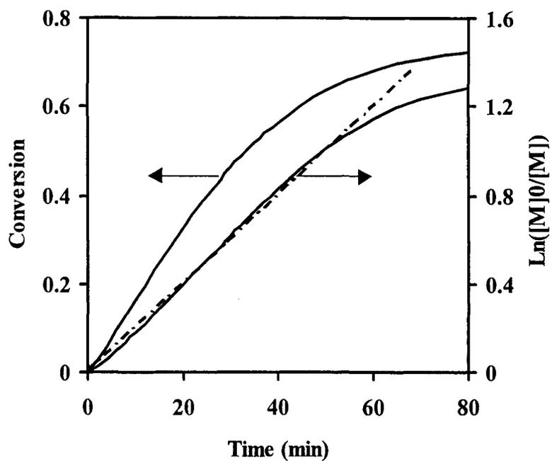
**Figure 2.3.** Kinetic curves for ATRP-1 of PEGDMA using the same reaction conditions as in Figure 2.2. The dash line indicates a linear portion of the  $\ln([M]_0/[M])$  vs time
