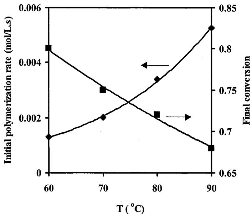
**Figure 2.15.** Effect of reaction temperature on the initial polymerization rate and the final vinyl group conversion in ATRP of PEGDMA:  $[\text{vinyl group}]_0 = 6.545 \text{ (mol/L)}$ ,  $[\text{MBPA}]_0 = [\text{CuBr}]_0 = [\text{HMATETA}]_0 = 0.06545 \text{ (mol/L)}$
