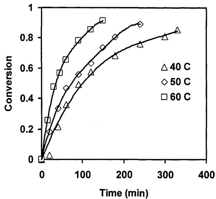
**Figure 3.2.** Monomer conversion of THF solution polymerization of DMAEMA vs time at 40, 50 and 60 °C with  $[\text{DMAEMA}]_0 = 2.96$  (mol/L) and  $[\text{ABIB}]_0 = [\text{CuBr}]_0 = [\text{PMDETA}]_0 = 0.0296$  (mol/L)
