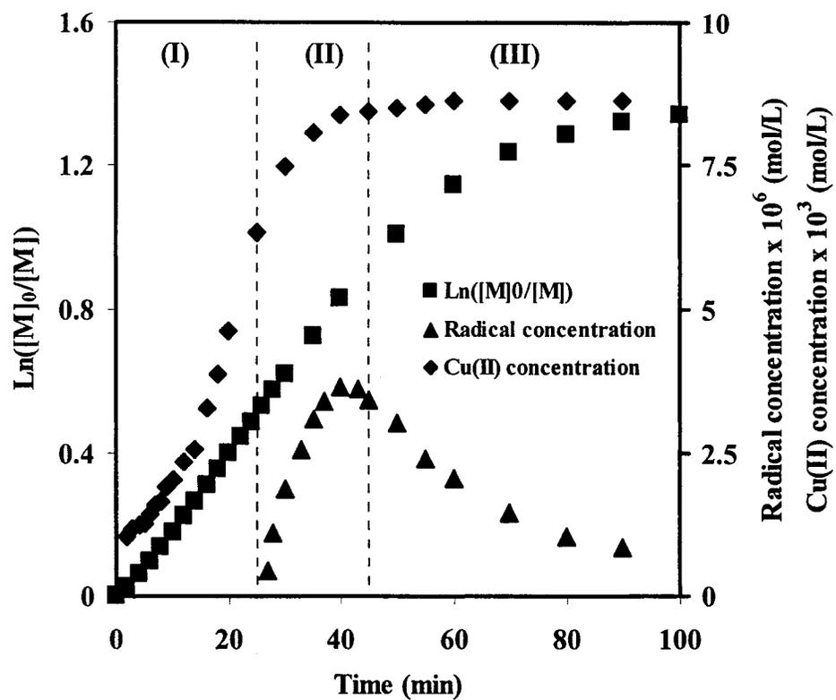
**Figure 2.11.**  $\text{Ln}([M]_0/[M])$ , radical concentration, and Cu(II) concentration vs polymerization time in the ATRP of PEGDMA at 70 °C:  $[\text{vinyl group}]_0 = 6.545 \text{ (mol/L)}$ ,  $[\text{MBPA}]_0 = [\text{CuBr}]_0 = [\text{HMATETA}]_0 = 0.06545 \text{ (mol/L)}$ .
