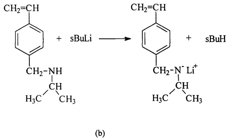
**Scheme B1.** Synthesis of N-isopropyl-4-vinylbenzylamine (a) and N-isopropyl-4-vinylbenzylamide (b)
