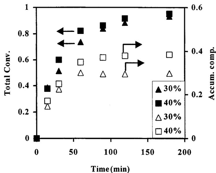
**Figure 5.13.** Total conversion and accumulative composition versus time for the semi-batch copolymerization of acrylamide with polyDMAEMA-DMS macromonomer in aqueous solution at 50 °C. Feeding policy: 0.8 g of acrylamide in 5% aqueous was initially charged to reactor; the macromonomer with initiator (0.2 g of polyDMAEMA-DMS and 10 mg of AIBA) in 5% solution was fed in a linearly decreasing mode from 0.075 mL/min to 0 mL/min in 2 h.
