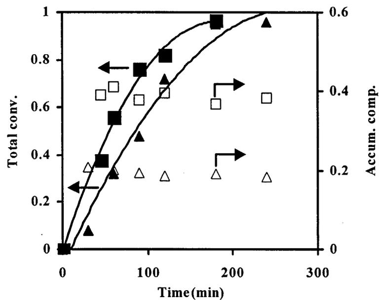
**Figure 5.14.** Total conversion and accumulative composition versus time for the semi-batch copolymerization of acrylamide with polyDMAEMA-DMS macromonomer in aqueous solution at 50 °C. Feeding policy: 0.8 g of acrylamide, 0.04 g of polyDMAEMA and 3 mg of AIBA in 5% aqueous was initially charged to reactor; the macromonomer with initiator (0.16 g polyDMAEMA-DMS, 7 mg of AIBA) was fed at a constant rate for 2 h.
