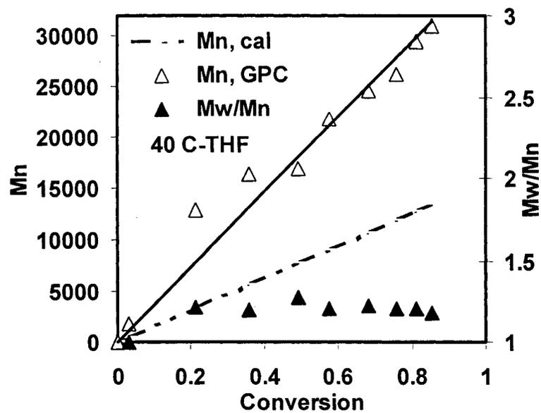
**Figure 3.6.** Molecular weight development of THF solution polymerization of DMAEMA at 40 °C with  $[\text{DMAEMA}]_0 = 2.96 \text{ M}$  and  $[\text{ABIB}]_0 = [\text{CuBr}]_0 = [\text{PMDETA}]_0 = 0.0296 \text{ M}$ . The molecular weights were measured by GPC.
