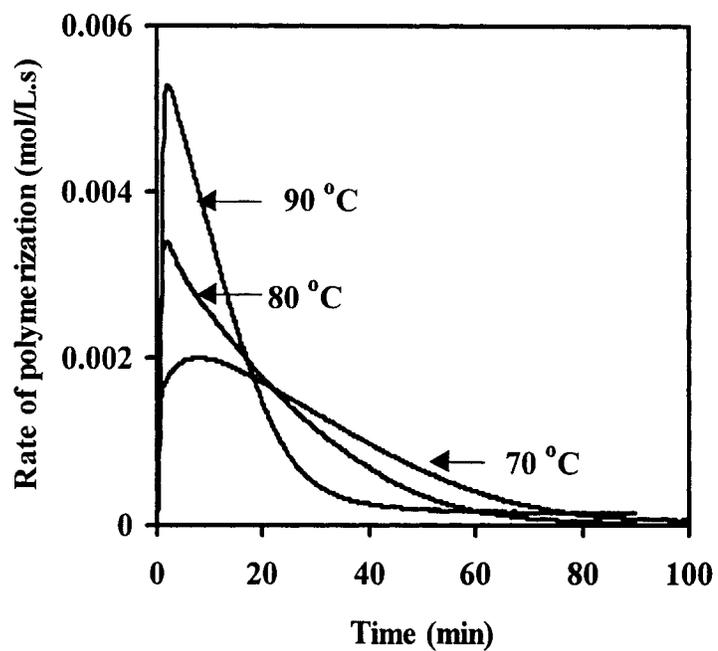
**Figure 2.14.** Polymerization rate profiles for the ATRP-1 system at different reaction temperatures:  $[\text{vinyl group}]_0 = 6.545 \text{ (mol/L)}$ ,  $[\text{MBPA}]_0 = [\text{CuBr}]_0 = [\text{HMATETA}]_0 = 0.06545 \text{ (mol/L)}$
