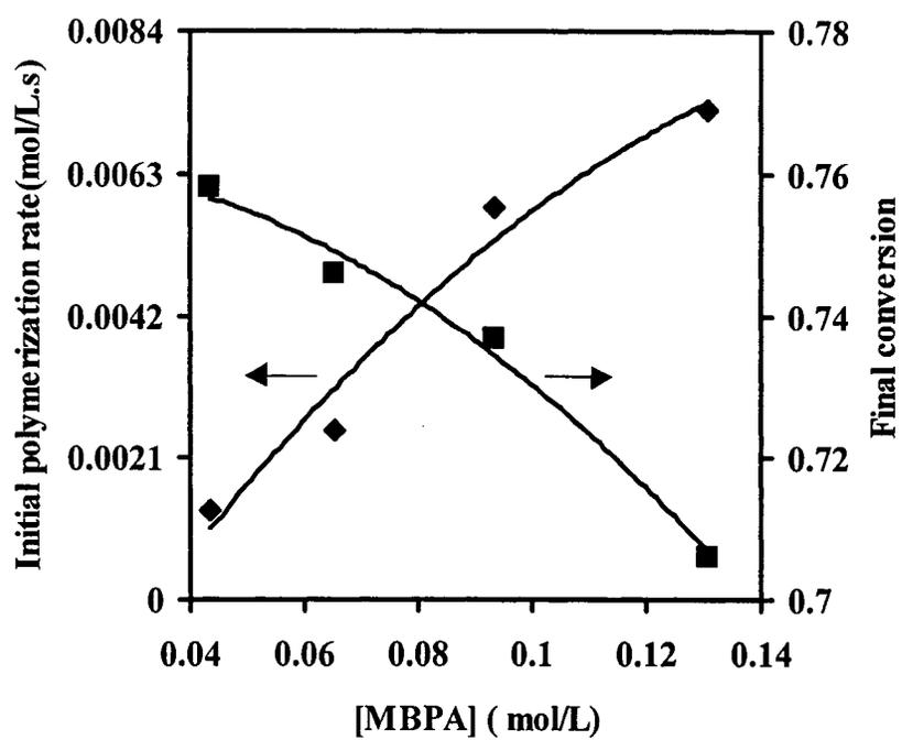
**Figure 2.13.** Influence of initiator concentration on the initial polymerization rate and the final vinyl group conversion in ATRP of PEGDMA at 70 °C:  $[\text{vinyl group}]_0 = 6.545$  (mol/L),  $[\text{MBPA}]_0/[\text{CuBr}]_0/[\text{HMATETA}]_0 = 1/1/1$
