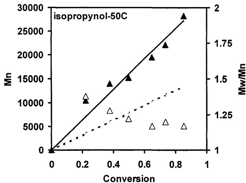
**Figure 3.10.** Number-average molecular weight and polydispersity versus conversion of isopropanol solution polymerization of DMAEMA at 60 °C with  $[\text{DMAEMA}]_0 = 2.96 \text{ M}$  and  $[\text{ABIB}]_0 = [\text{CuBr}]_0 = [\text{PMDETA}]_0 = 0.0296 \text{ M}$ .  $M_{n, \text{GPC}}$
