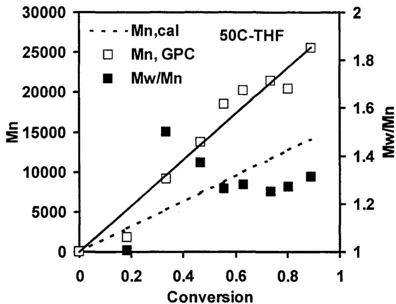
**Figure 3.5.** Molecular weight development of THF solution polymerization of DMAEMA at 50 °C with  $[\text{DMAEMA}]_0 = 2.96 \text{ M}$  and  $[\text{ABIB}]_0 = [\text{CuBr}]_0 = [\text{PMDETA}]_0 = 0.0296 \text{ M}$ , The molecular weights were measured by GPC.
