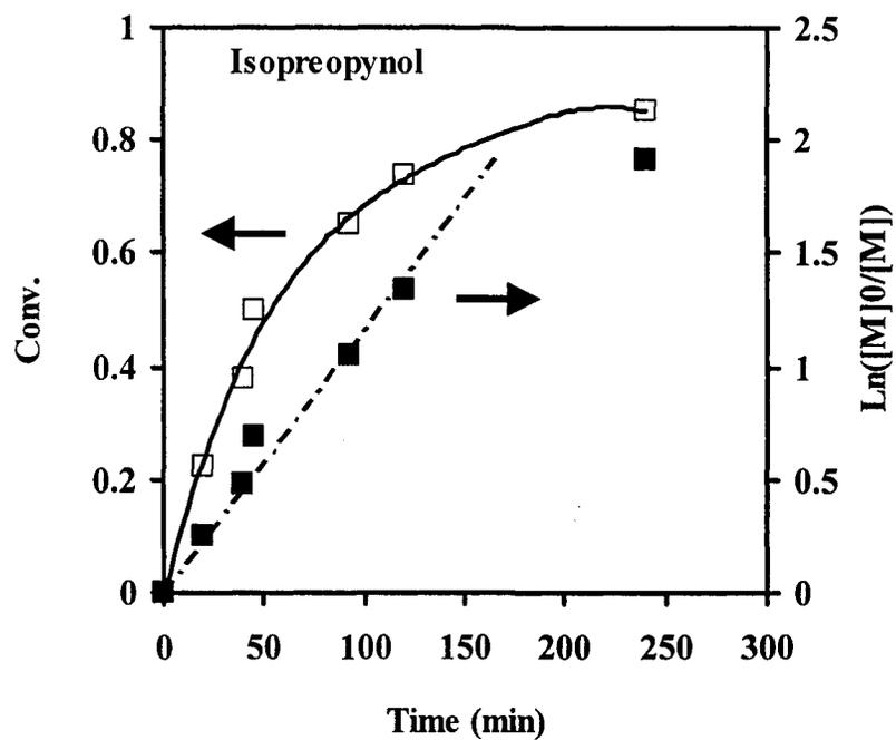
**Figure 3.9** Monomer conversion and  $\ln([M]_0/[M])$  versus time of isopropanol solution polymerization of DMAEMA at 60 °C with  $[DMAEMA]_0 = 2.96$  M and  $[ABIB]_0 = [CuBr]_0 = [PMDETA]_0 = 0.0296$  M.
