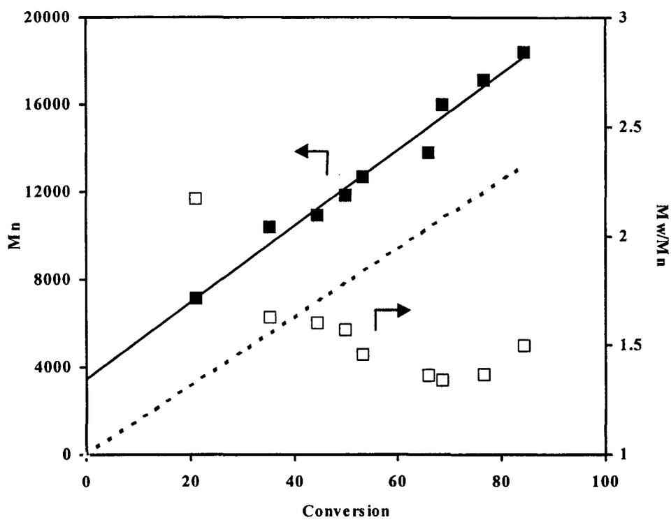
**Figure A5.** Molecular weight of poly(DMAEMA) as a function of conversion in aqueous ATRP of DMAEMA. See Figure 4 for conditions.
