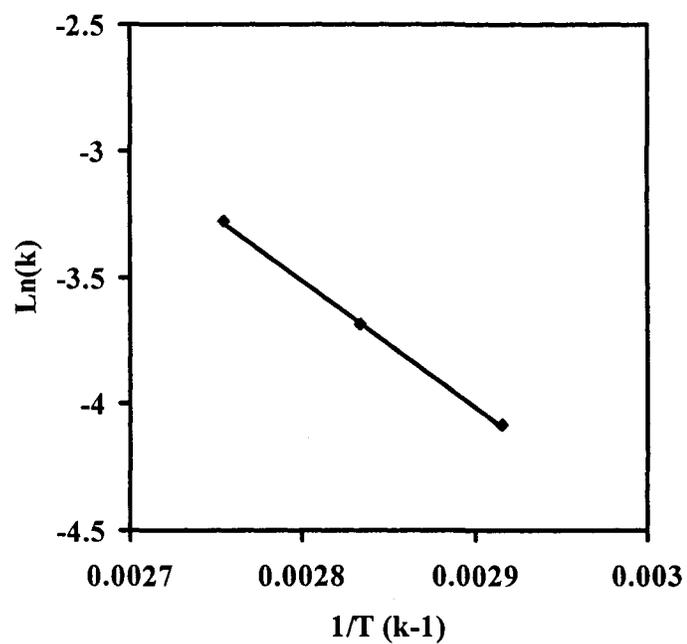
**Figure 2.16.** Arrhenius plot of the ATRP of PEGDMA using the same reaction conditions as in Figure 2.14.
