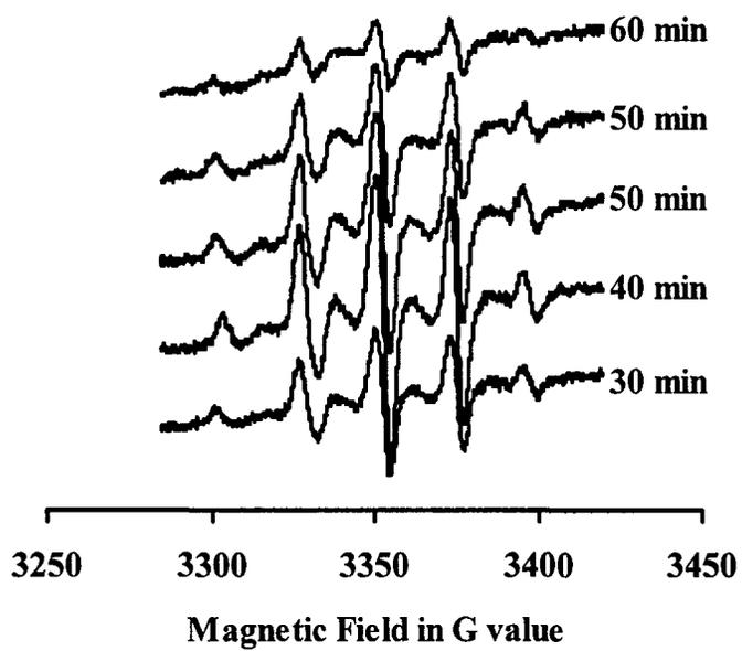
**Figure 2.9** ESR signals from methacrylate radicals in the ATRP process of PEGDMA using the same reaction conditions as in Figure 2.8
