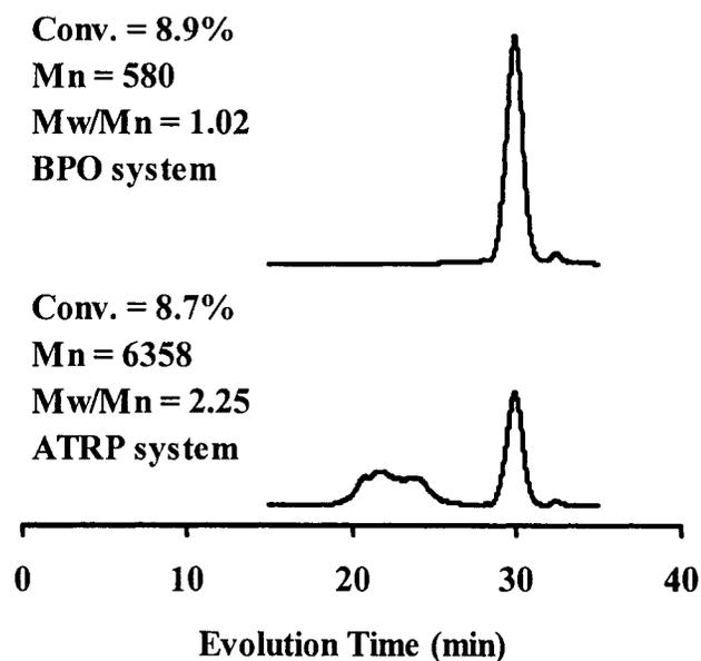
**Figure 2.4.** GPC curves for sol. fractions from BPO and ATRP-1 reaction systems at 70 °C.
