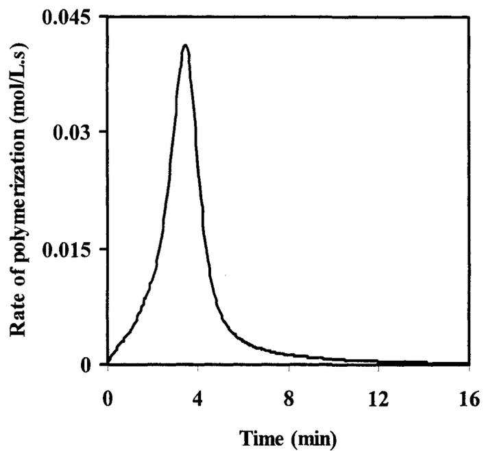
**Figure 2.1.** Polymerization rate profile for the BPO-initiated polymerization of PEGDMA at 70 °C:  $[\text{vinyl group}]_0 = 6.545 \text{ (mol/L)}$ ,  $[\text{BPO}]_0 = 0.06545 \text{ (mol/L)}$
