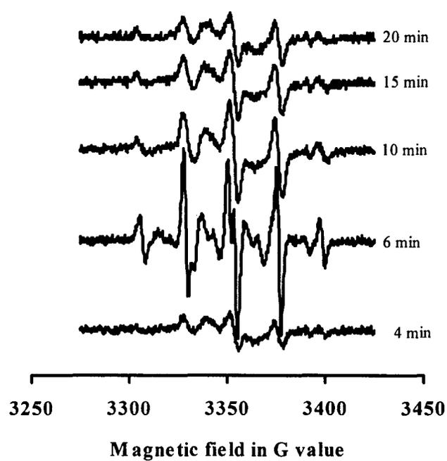
**Figure 2.6.** ESR spectra recorded during the BPO-initiated polymerization of PEGDMA at 70 °C:  $[\text{vinyl group}]_0 = 6.545 \text{ (mol/L)}$ ,  $[\text{BPO}]_0 = 0.06545 \text{ (mol/L)}$ .
