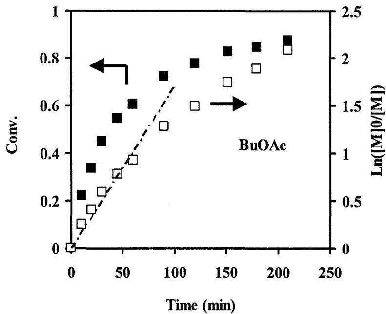
**Figure 3.7** Monomer conversion and  $\ln([M]_0/[M])$  vs time of n-butyl acetate solution polymerization of DMAEMA at 60 °C with  $[DMAEMA]_0 = 2.96$  M and  $[ABIB]_0 = [CuBr]_0 = [PMDETA]_0 = 0.0296$  M.
