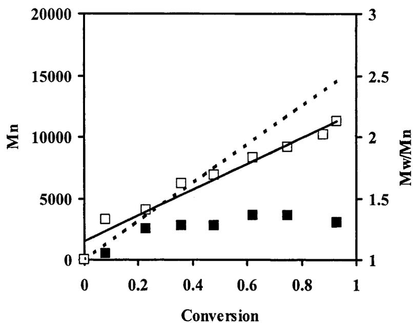
**Figure 3.12.** Number-average molecular weight and polydispersity versus conversion of THF solution polymerization of DMAEMA at 60 °C with  $[\text{DMAEMA}]_0 = 2.96 \text{ M}$  and  $[\text{ABIB}]_0 = [\text{CuBr}]_0 = [\text{BA}_6\text{-TREN}]_0 = 0.0296 \text{ M}$ .  $M_{n,\text{GPC}}$  ( $\square$ ),  $M_{n,\text{cal}}$  (---),  $M_w/M_n$  ( $\blacksquare$ ).
