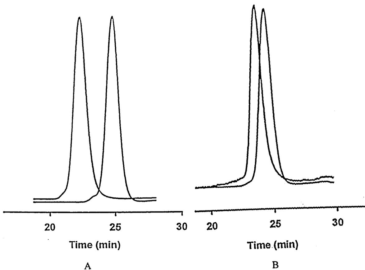
Figure B1. SEC traces for poly(DMAEMA-*block*-MMA) and poly(tBMA-*block*-MMA) synthesized by a two-step process with LiPVBA initiator: A) prepolymer,  $M_n = 3,340$ ; block,  $M_n = 11,340$  (Table 2, entry 8); B) prepolymer:  $M_n = 3,600$ ; block copolymer,  $M_n = 5,400$  (Table B2, entry 10).
