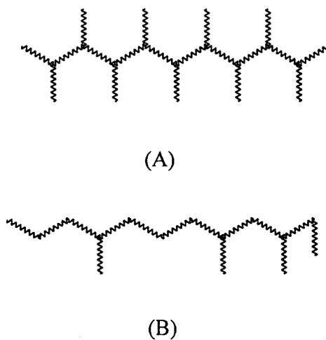
**Figure 5.12.** Graft copolymers: (A) homogeneous graft copolymer; (B) heterogeneously grafted copolymer
