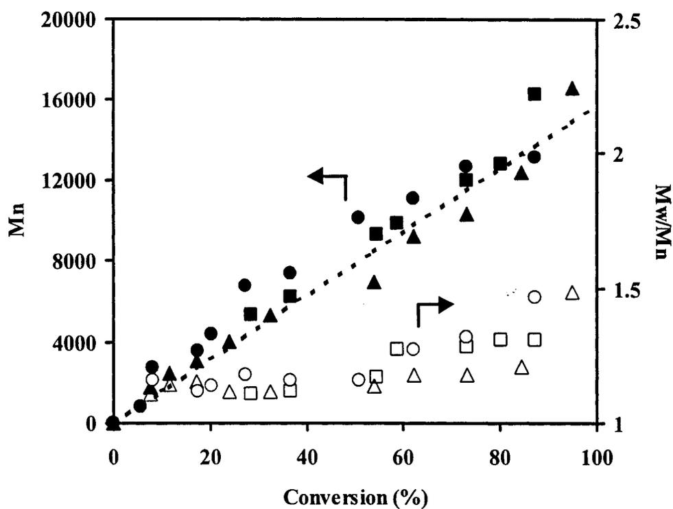
**Figure A3.** Molecular weight of poly(DMAEMA) as a function of conversion in aqueous
