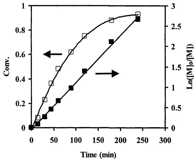
**Figure 3.11.** Monomer conversion and  $\ln([M]_0/[M])$  versus time of THF solution polymerization of DMAEMA at 60 °C with  $[DMAEMA]_0 = 2.96$  M and  $[ABIB]_0 = [CuBr]_0 = [BA_6-TREN]_0 = 0.0296$  M.
