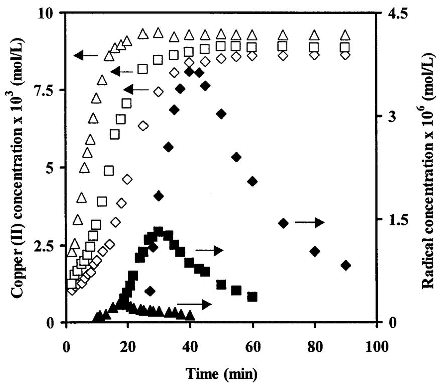
**Figure 2.10.** Copper (II) and radical concentrations as functions of reaction time for ATRP-1 system at different reaction temperatures:  $[\text{vinyl group}]_0 = 6.545 \text{ (mol/L)}$ ,  $[\text{MBPA}]_0 = [\text{CuBr}]_0 = [\text{HMTETA}]_0 = 0.06545 \text{ (mol/L)}$ : ( $\diamond$ ,  $\blacklozenge$ ) 70, ( $\square$ ,  $\blacksquare$ ) 80 and ( $\blacktriangle$ ,  $\triangle$ ) 90 °C
