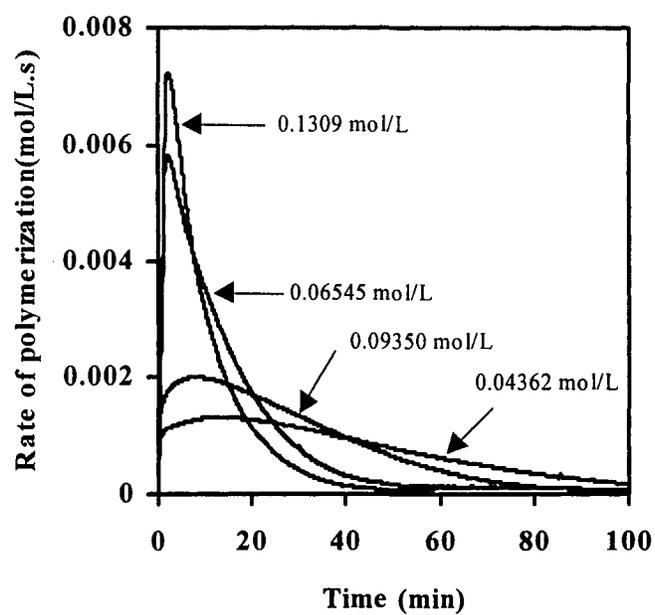
**Figure 2.12.** Polymerization rate profiles for ATRP of PEGDMA with different initiator concentrations at 70 °C:  $[\text{vinyl group}]_0 = 6.545 \text{ (mol/L)}$ ,
