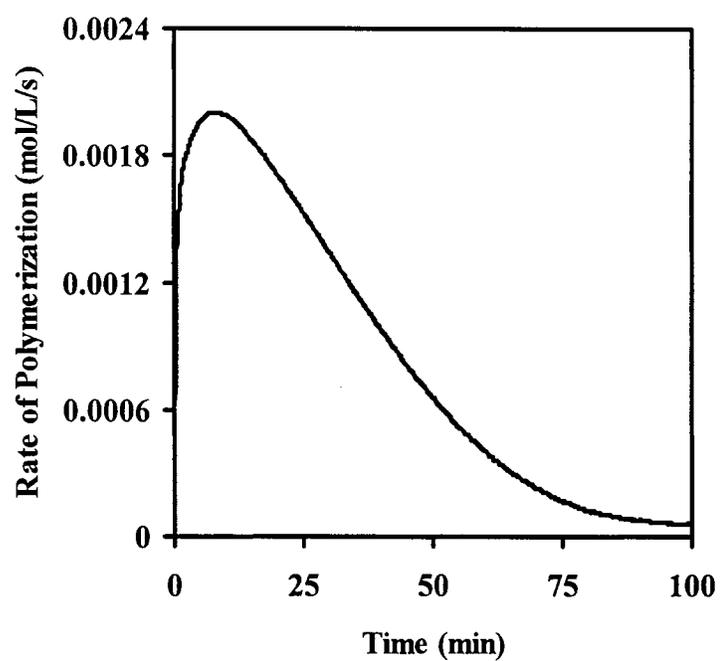
**Figure 2.2.** Polymerization rate profile for the ATRP-1 of PEGDMA at 70 °C:
