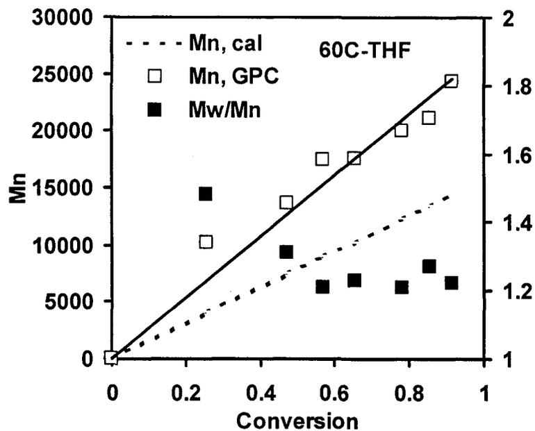
**Figure 3.4** Molecular weight development of THF solution polymerization of DMAEMA at 60 °C with  $[\text{DMAEMA}]_0 = 2.96 \text{ M}$  and  $[\text{ABIB}]_0 = [\text{CuBr}]_0 = [\text{PMDETA}]_0 = 0.0296 \text{ M}$ . The molecular weights were measured by GPC.
