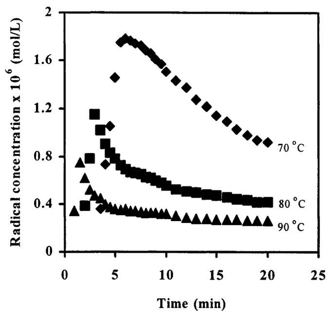
**Figure 2.7.** Variation of radical concentration measured by ESR during the BPO-initiated polymerization of PEGDMA at different temperatures:  $[\text{vinyl group}]_0 = 6.545$  (mol/L),  $[\text{BPO}]_0 = 0.06545$  (mol/L).
