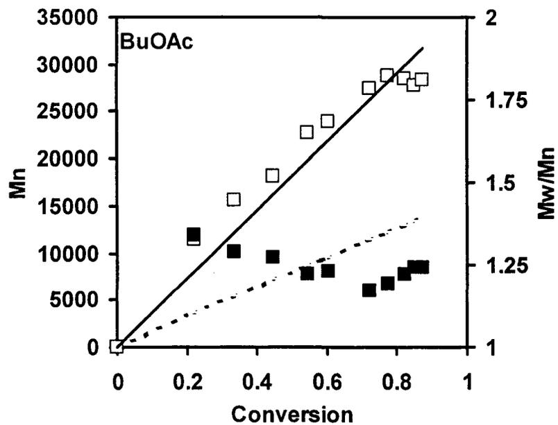
**Figure 3.8** Number-average molecular weight and polydispersity versus conversion of n-butyl acetate solution polymerization of DMAEMA at 60 °C with  $[\text{DMAEMA}]_0 = 2.96 \text{ M}$  and  $[\text{ABIB}]_0 = [\text{CuBr}]_0 = [\text{PMDETA}]_0 = 0.0296 \text{ M}$ .  $M_{n,\text{GPC}}$  ( $\square$ ),  $M_{n,\text{cal}}$  (---),  $M_w/M_n$  ( $\blacksquare$ ).
