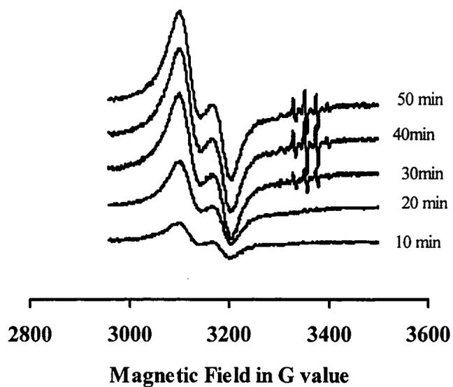
**Figure 2.8** ESR spectra recorded during the ATRP process of PEGDMA at 70 °C:
