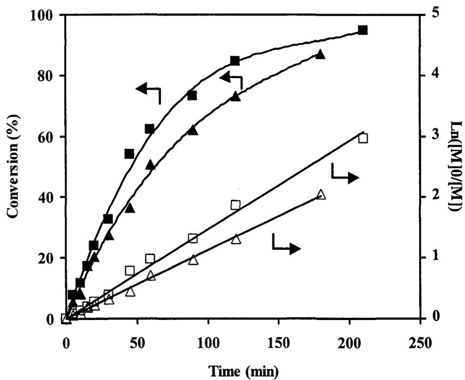
**Figure A2.** The aqueous ATRP of DMAEMA catalyzed by CuBr-Bpy at 20 °C at different catalyst concentration.  $[\text{DMAEMA}]_0/[\text{MBP}]_0/[\text{CuBr}]_0/[\text{Bpy}]_0 = 100:1:1:2$  (in mole) (■, □),  $[\text{DMAEMA}]_0/[\text{MBP}]_0/[\text{CuBr}]_0/[\text{Bpy}]_0 = 100:1:0.5:1$  (in mole) (▲, △)
