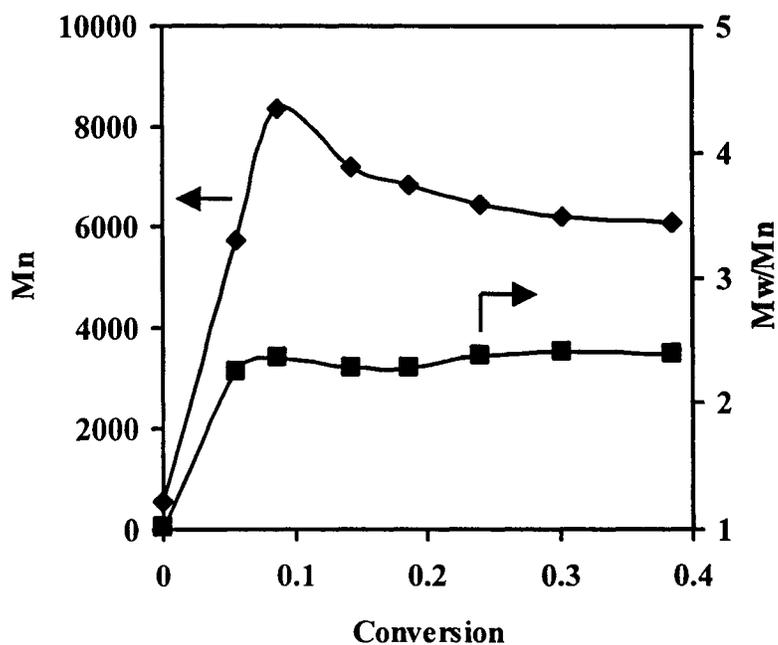
**Figure 2.5.** Variation of molecular weight and molecular weight distribution of sol polymer with vinyl group conversion for ATRP-1 at 70 °C.
