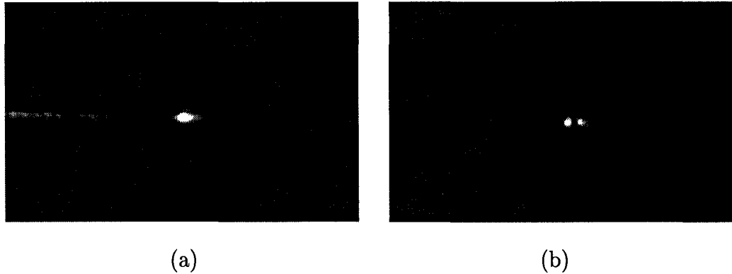
Figure 5.4: Near field camera images of TE waveguide modes for a 5\ \mu\text{m} ridge width: (a) excitement of the first order mode (b) excitement of the second order mode.
