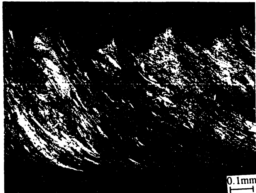
Fig. 4.49(a): Optical micrograph of a continuous chip obtained at a cutting speed of 350 m/min., during machining of Fe-1.4%Ni-0.1%C alloy. The dark band is the region that undergoes phase transformation from martensite to austenite and back to refined martensite.
