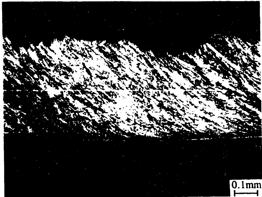
Fig. 4.48(a): Optical micrograph of a continuous chip obtained at a cutting speed of 250 m/min., during machining of Fe-1.4%Ni-0.1%C alloy. The dark band is the region that undergoes phase transformation from martensite to austenite and back to refined martensite.
