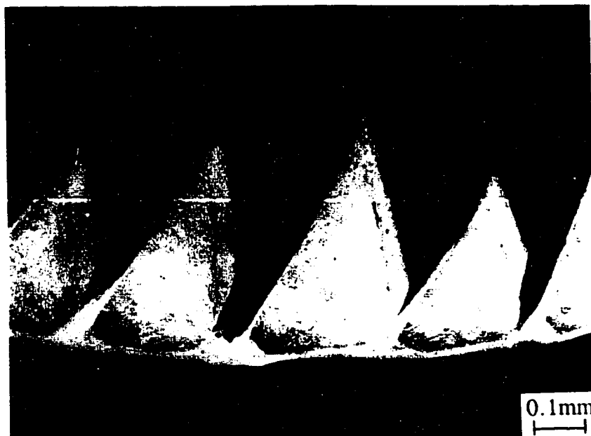
Fig. 4.63(a): Optical micrograph of a fully segmented chip obtained at a feed of 0.397 mm/rev and a cutting speed of 350 m/min in Fe-18.9%Ni-0.10%C.
