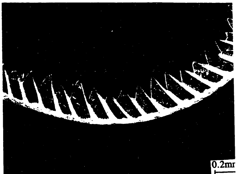
Fig. 4.74(a): Optical micrograph of a fully segmented chip obtained at a cutting speed of 300 m/min. With use of coolant, showing transformation shear band enveloping the segmented chip at cutting speed of 300 m/min in Fe-28.9wt%Ni-0.1wt%C alloy. The white region that has undergone phase transformation from martensite to austenite at 400°C.
