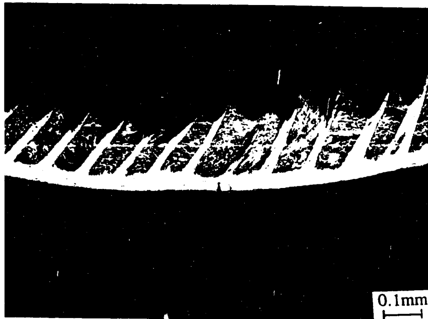
Fig. 4.56(a): Optical micrograph of a fully segmented chip obtained at a feed of 0.206 mm/rev and a cutting speed of 400 m/min in Fe-28.9%Ni-0.10%C.
