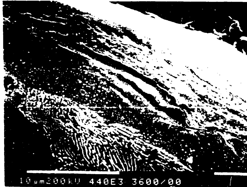
Fig. 4.10(e): SEM image of the chip segments machined from ductile iron using a cemented carbide tool (K1) at 300 m/min, showing a deformation shear band in which the graphite spheroid is extruded into a very thin slab indicating large strain in the shear band.
