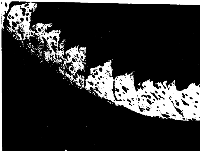
Fig. 4.10(b): An optical micrograph showing a section parallel to the chip flow direction of a partially segmented chip obtained from machining ductile iron with cemented carbide tool (K1) at a cutting speed of 200 m/min. Etched in 2% nital. (Mag.50X)
