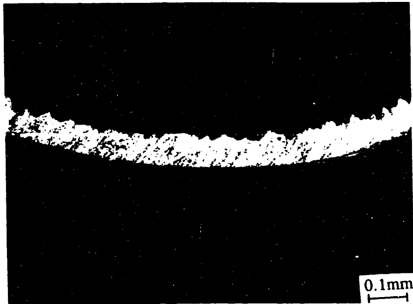
Fig. 4.64(a): Optical micrograph of a continuous or flow chip obtained at a feed of 0.055 mm/rev and a cutting speed of 400 m/min in Fe-9.7%Ni-0.10%C.
