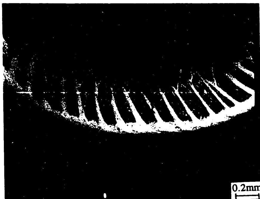
Fig. 4.73(a): Optical micrograph of a fully segmented chip obtained at a cutting speed of 150 m/min. And with use of a coolant, showing transformation shear band enveloping the segmented chip at cutting speed of 150 m/min in Fe-28.9wt%Ni-0.1wt%C alloy. The white region that has undergone phase transformation from martensite to austenite at 400°C.
