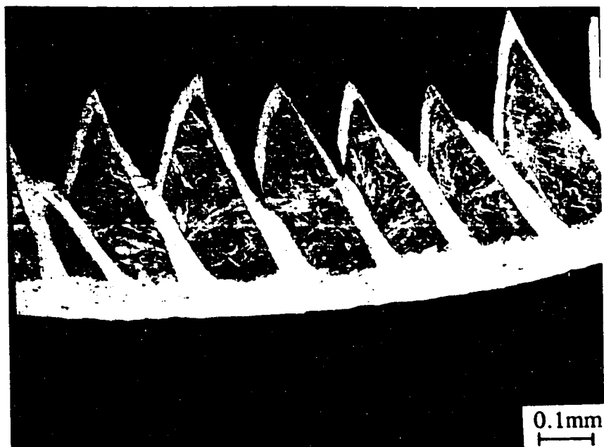
Fig. 4.70(a): Optical micrograph of a fully segmented chip obtained at a cutting speed of 300 m/min. and a depth of cut of 2.0 mm, showing transformation shear band enveloping the segmented chip obtained from an Fe-28.9wt%Ni-0.1wt%C alloy. The white band is the region that has undergone phase transformation from martensite to austenite at 400°C.
