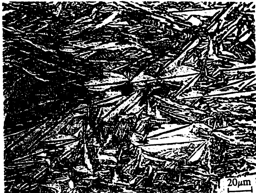
Fig. 3.6: Optical micrograph showing the microstructure of martensite in quenched Fe-28.9%Ni-0.10%C alloy before machining.
