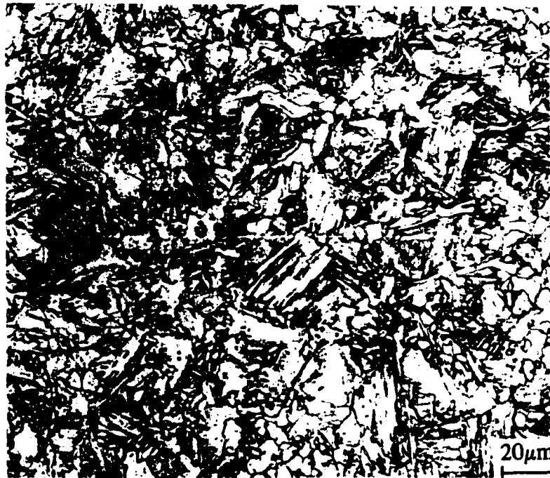
Fig. 3.9: Optical micrograph showing the microstructure of quenched Fe-1.4%Ni-0.10%C alloy before machining, with evidence of ferrite, pearlite and islands of martensite.
