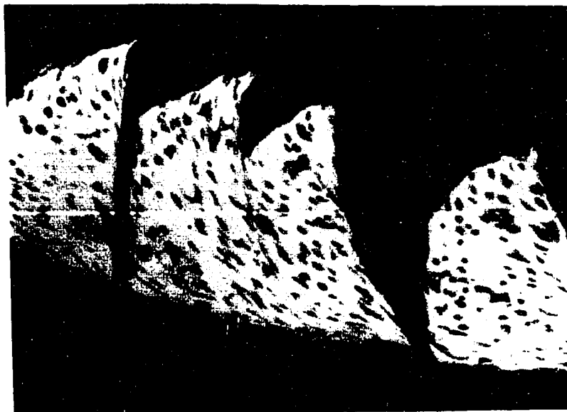
Fig. 4.10(c): An optical micrograph showing a section parallel to the chip flow direction of the chip obtained from machining ductile iron with cemented carbide tool (K1) at a cutting speed of 300 m/min, showing partial separation of the segments. Etched in 2% nital. (Mag. 50X)
