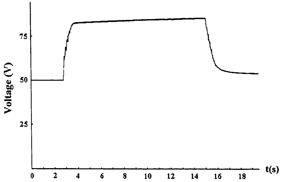
Figure 3.27 Energy storage tank voltage (10A test)
