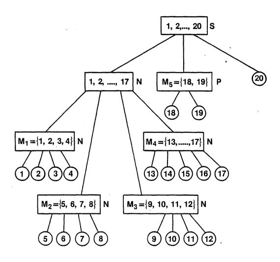
A poset P and its decomposition tree with the type indicators beside each internal node.
