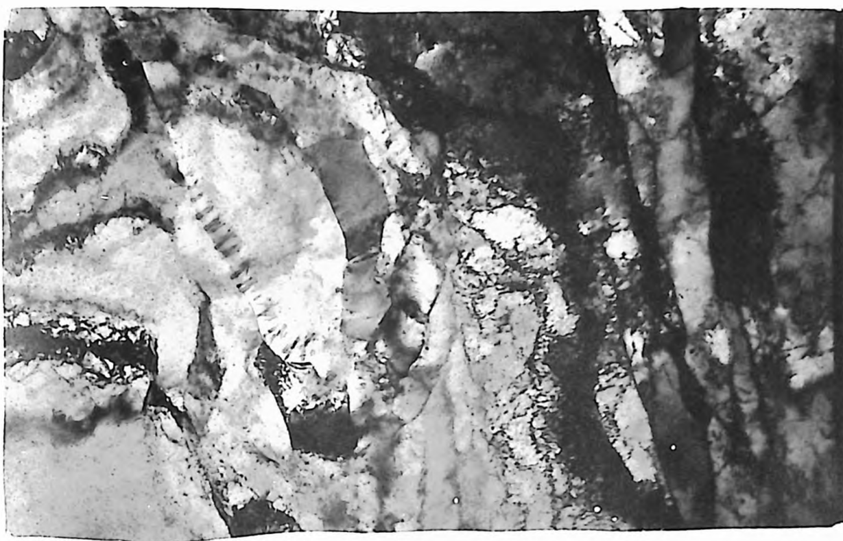
Fig. 38 Refinement of cell structure. \times 40,000
