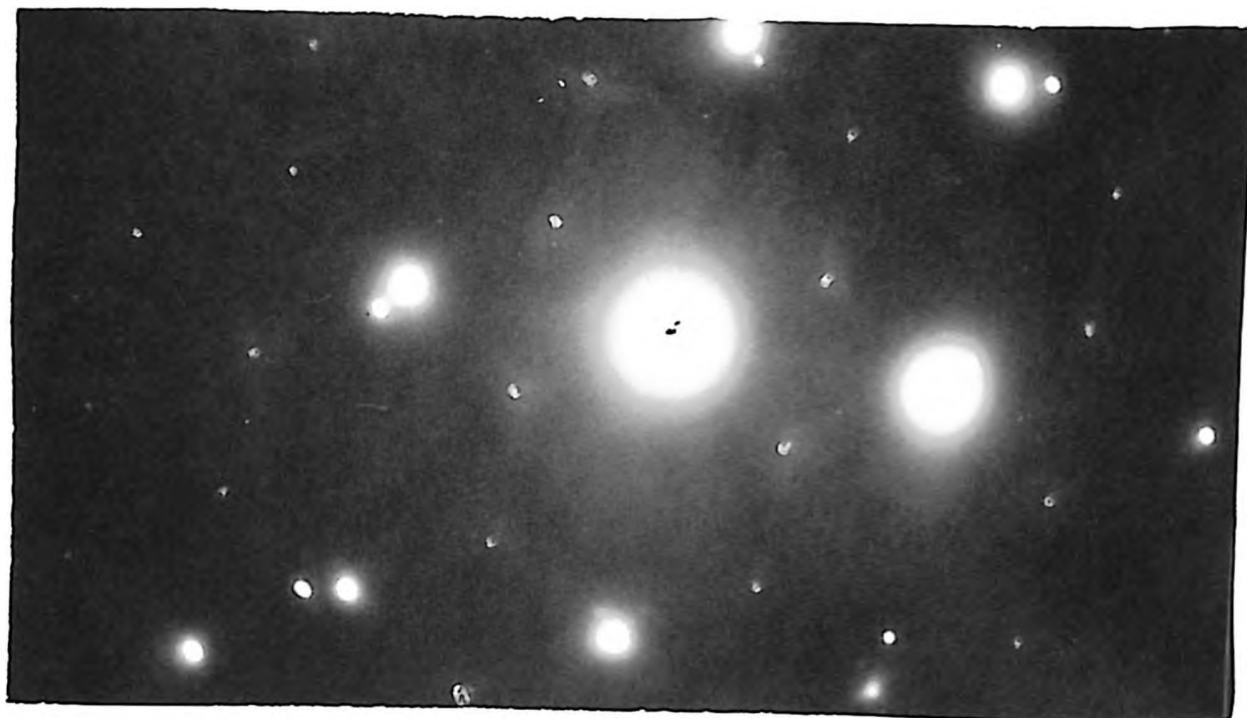
Fig. 7 Diffraction pattern of dark lamellae in figure 6. (foil normal [\bar{1}11] )
