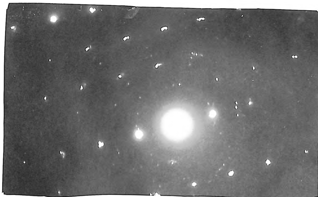
Fig. 8 Diffraction pattern of matrix in figure 6 ( foil normal [\bar{1}21] )
