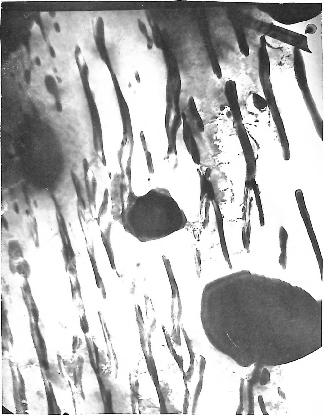
Fig. 6 Slow cooled Superston Bronze, coarsening of random lamellae. X3,500
