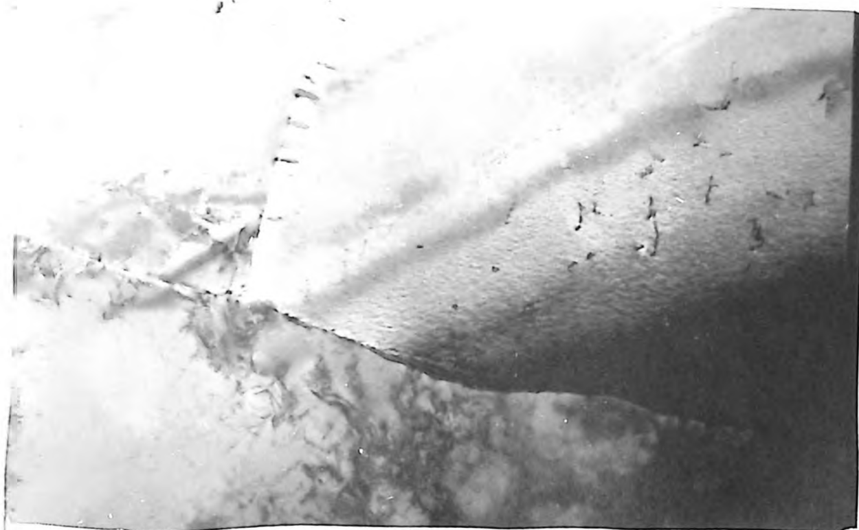
Fig. 33 Heterogeneous precipitate. X40,000
