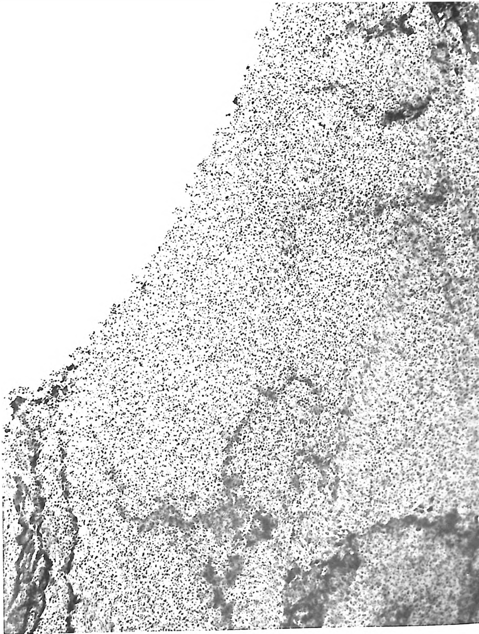
Fig. 42 Precipitate present after fatigue. X102,000
