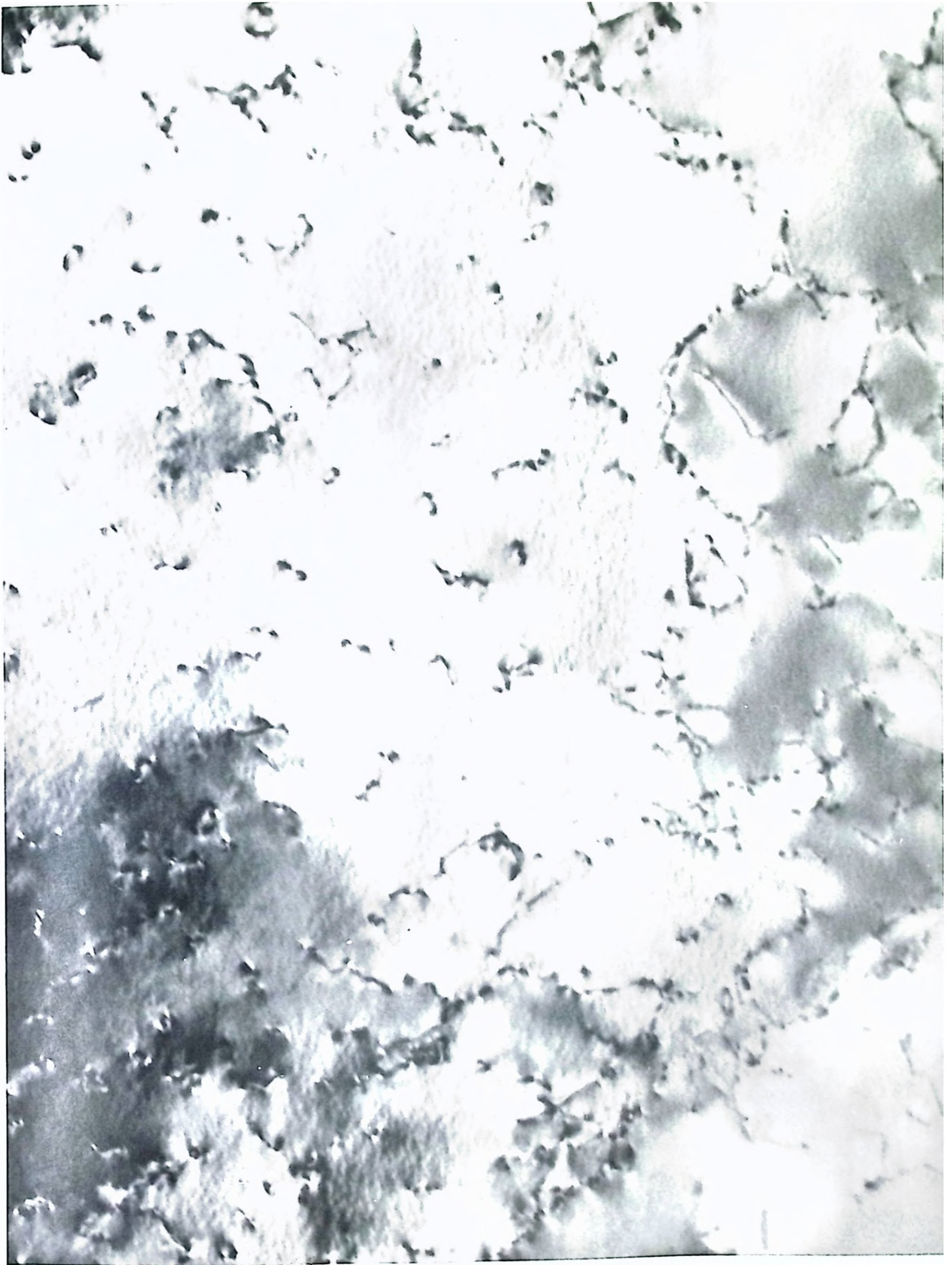
Fig. 27 Dislocation substructure within coarse cells.
