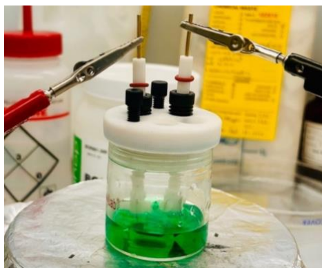
Figure 3.5. The design of sealed electrolytic cell.
