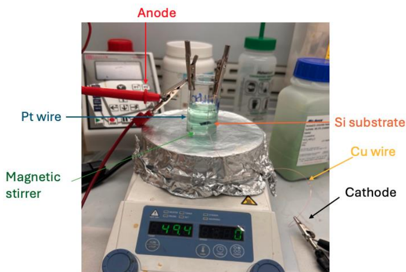
Figure 3.2. The design of wrapping Si substrate with Cu wire in a beaker. Alligator clips were used to provide stability and establish electrical connection with the power supply.
