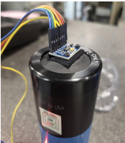
Figure 19: ADXL-345 mounted on shaker
