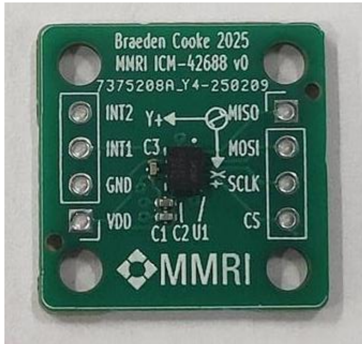
Figure 11: ICM-42688-P Evaluation PCB (0.8" x 0.8")
