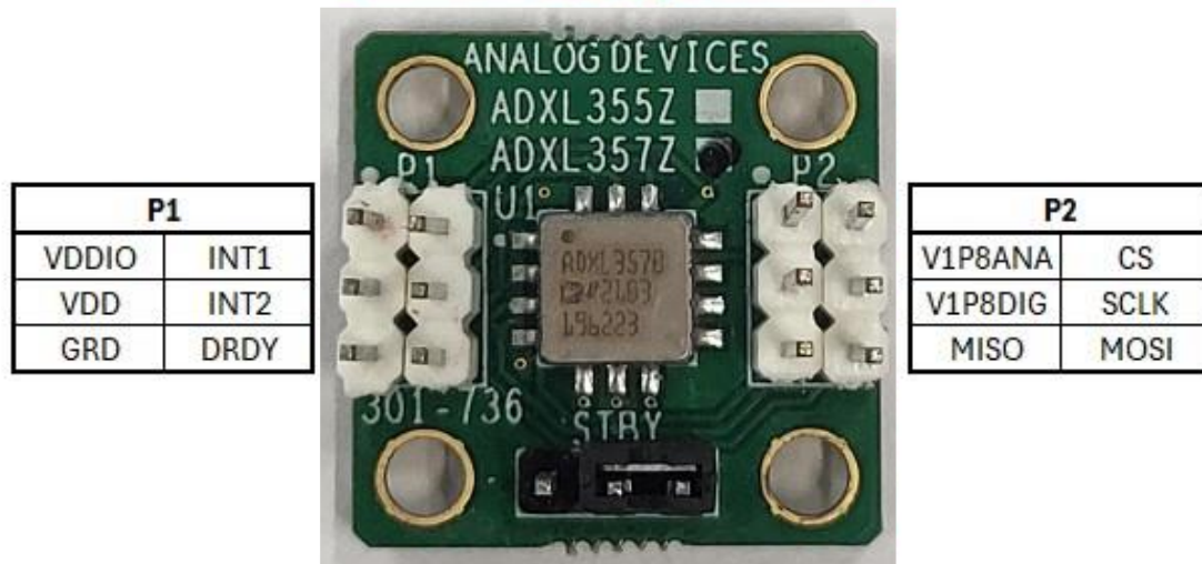
Figure 10: EVAL-ADXL-357Z PCB (0.8" x 0.8")
