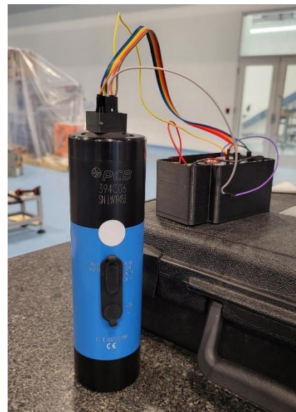
Figure 20: ADXL-357 mounted on shaker
