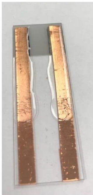
Figure S1. Photograph of a fabricated chemiresistive sensing device.
