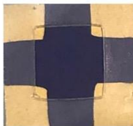
Figure S2. Photographic image of \text{SiO}_2 substrate ( 1 \times 1 \text{ cm}^2 ) with gold contacts in the four corners for the four-probe measurement.
