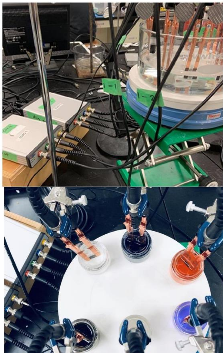
Figure S36. Experimental setup of the experiment (top) and functionalization of the sensors with redox-active molecules (bottom). The molecule solutions exhibit the following coloration: PCAT appears as a deep blue, APCAT appears as red, LCV is a pale blue, DPPD is a deep black, and DPB is white.
