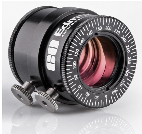
Figure 2.21: TECHSPEC Risley Prism Mount from Edmund Optics, enabling beam steering through independent rotation of two wedge prisms [97].
