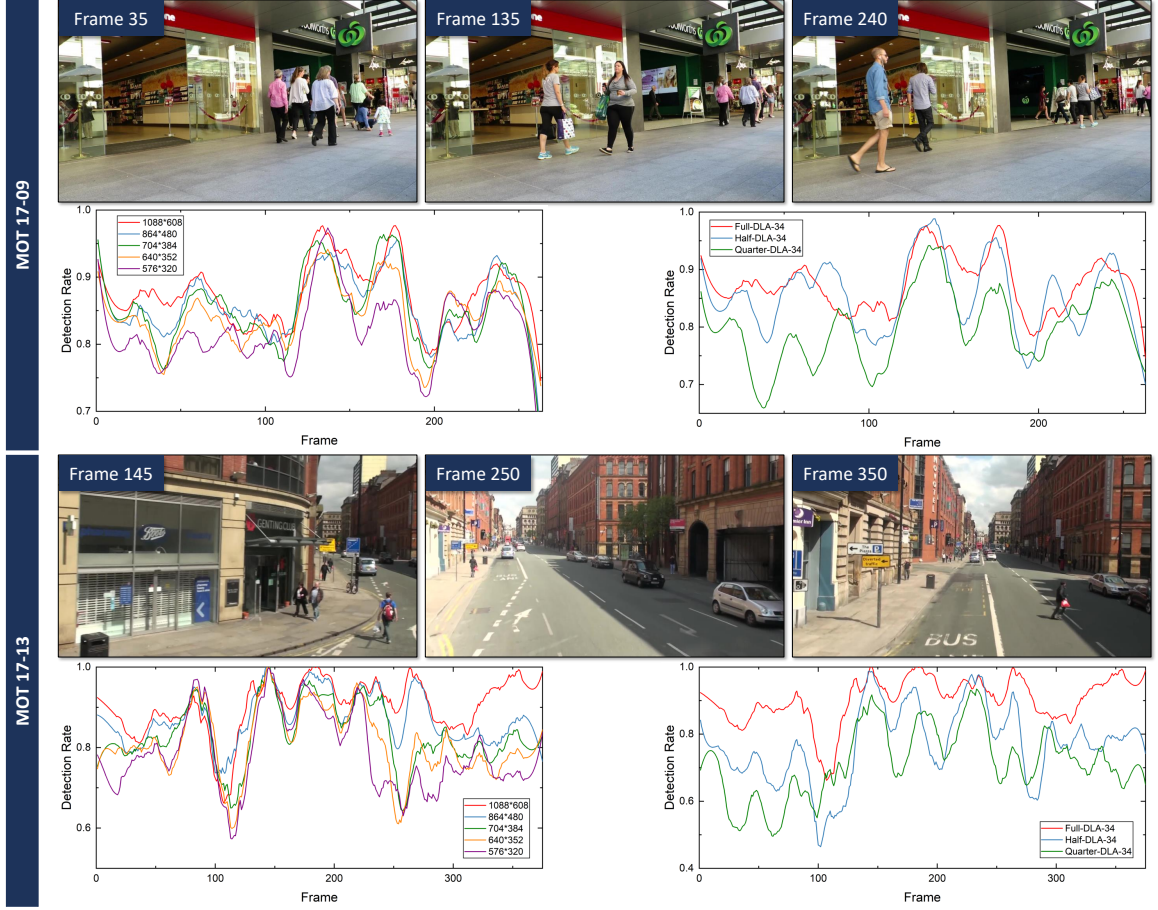
Figure 3.1: Detection rate using FairMOT with different input resolutions and backbone models on two video sequences of MOT17 dataset.
