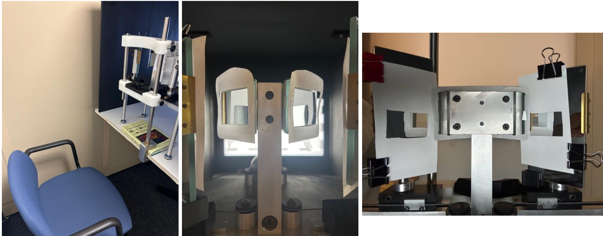
Figure B1 Pictured on the left is the participant seating and chin rest setup. Pictured next are the innermost mirrors on the mirror stereoscope. The metal edges of the mirrors have been covered with white paper. On the right are the two large outer mirrors of the stereoscope. The mirrors have been covered with sheets of paper with a rectangle cut out in the centre to restrict participants' view to the monitor.
