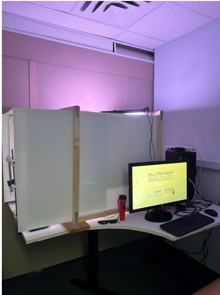
Figure B2 The first version of the enclosure was built with a wooden frame. White corrugated plastic sheets were placed on the inside to create an enclosure surrounding the setup. White Bristol board was adhered onto the plastic sheets to eliminate reflections from the monitor.
