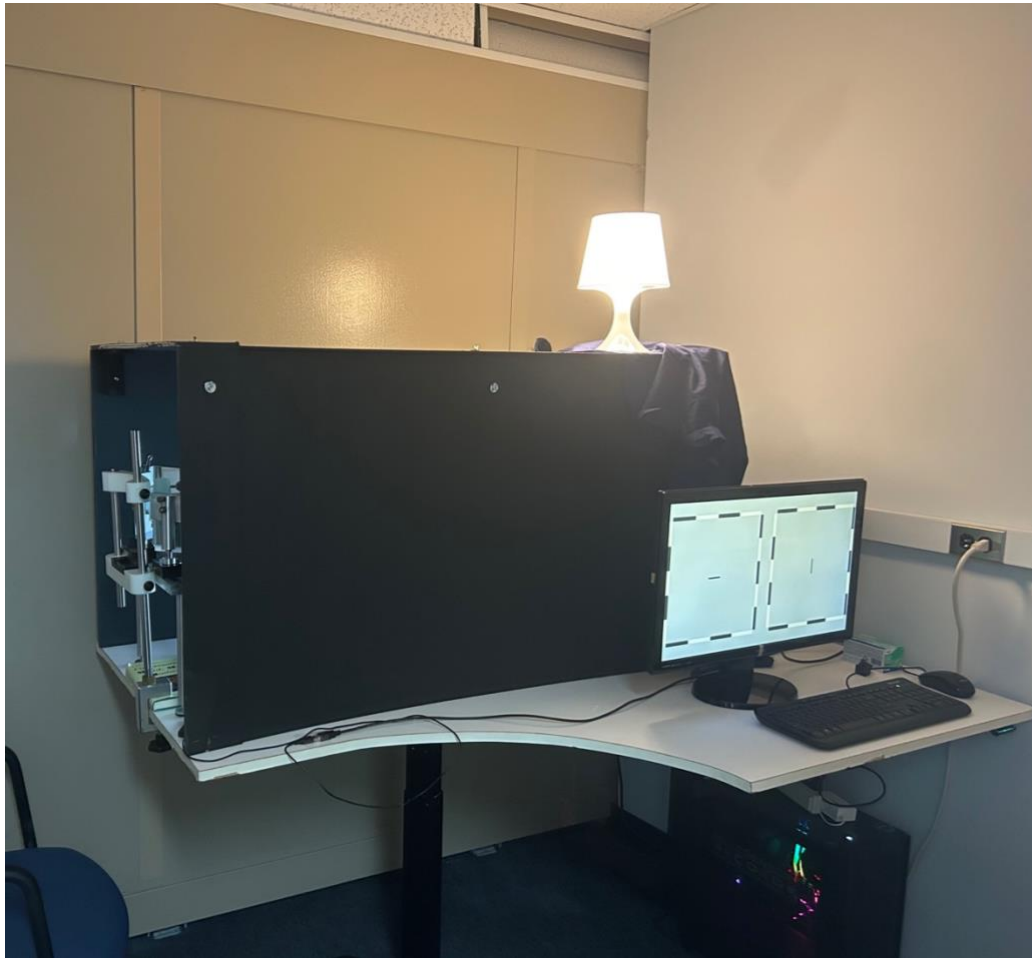
Figure B3 The second version of the enclosure was built with plywood that was then painted black and attached using L brackets.
