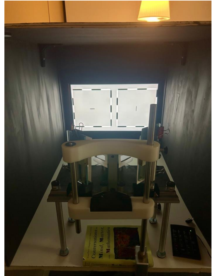
Figure B3 The second version of the enclosure was built with plywood that was then painted black and attached using L brackets.
