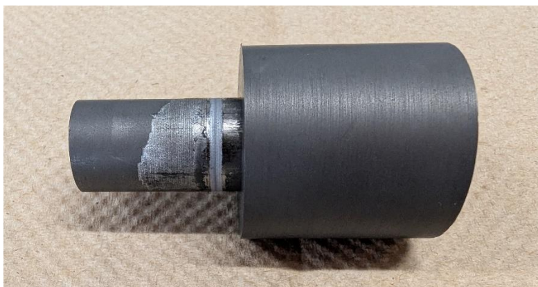
Figure S1.4b. Photograph of the cadmium leakage from the SPS graphite die/punch.
