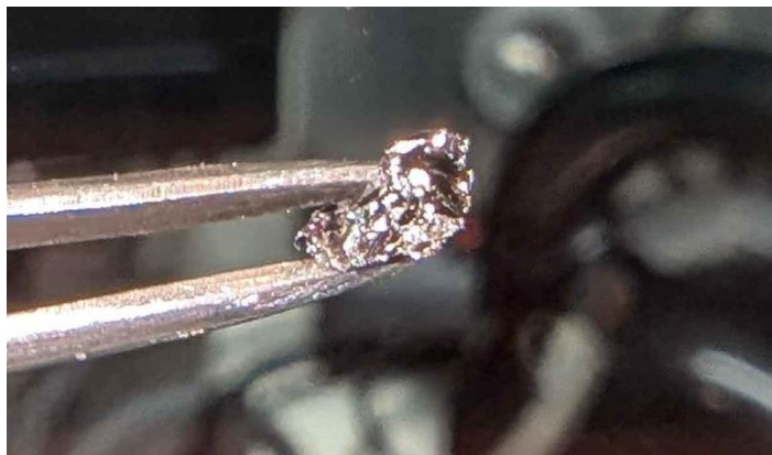
Figure S1.2b. Photograph of the KSb crystal inside the Ar-filled glovebox.
