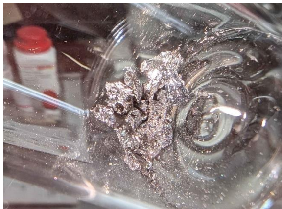
Figure S1.2a. Photograph of the KSb polycrystalline precursor extracted from the carbon-coated quartz tube inside the Ar-filled glovebox.
