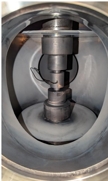
Figure S1.4a. Photograph of a cadmium-covered walls inside the SPS chamber. The clean chamber is shiny. The dull grey deposit is elemental cadmium.
