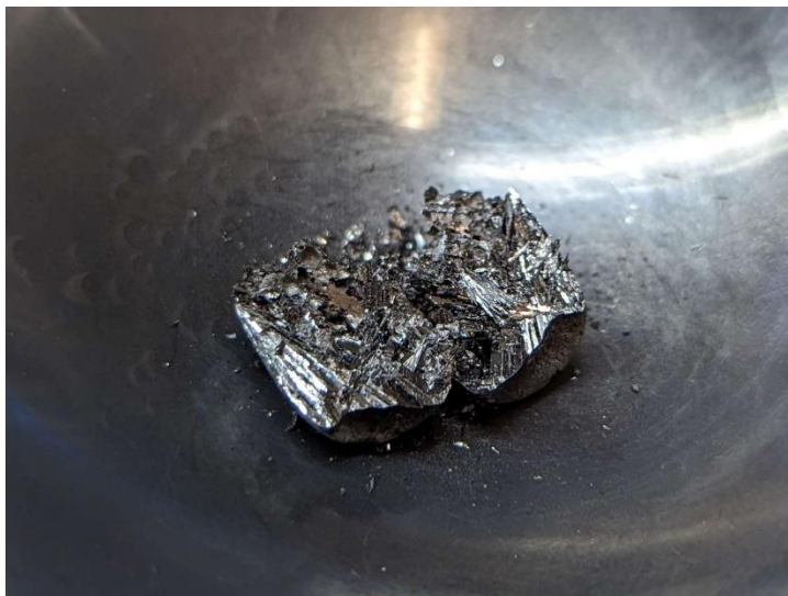
Figure S1.1. Photograph of the NaSb polycrystalline precursor inside of an Ar glovebox. Needle-shaped crystals are visible on the surface.
