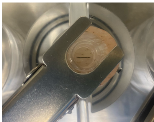
Figure 2.2: Franz diffusion cell components (left); a bird's eye view of the skin prior to lead application (right). Skin is positioned such that the hair (the black line at the center of the image) is aligned with the donor and receptor chamber openings.
