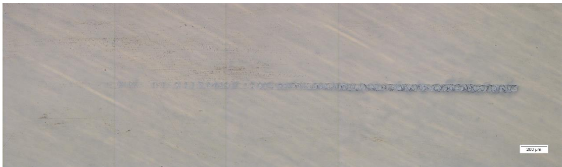
Figure 5. 3 Optical image of SiC surface scratched by a gradient force 1-30 N. Error! B
