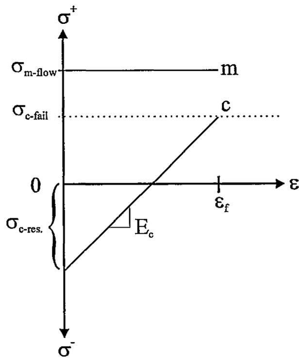
Figure 6.4: Schematic of proposed flow and fracture response of Ni:TZ8Y composites.
