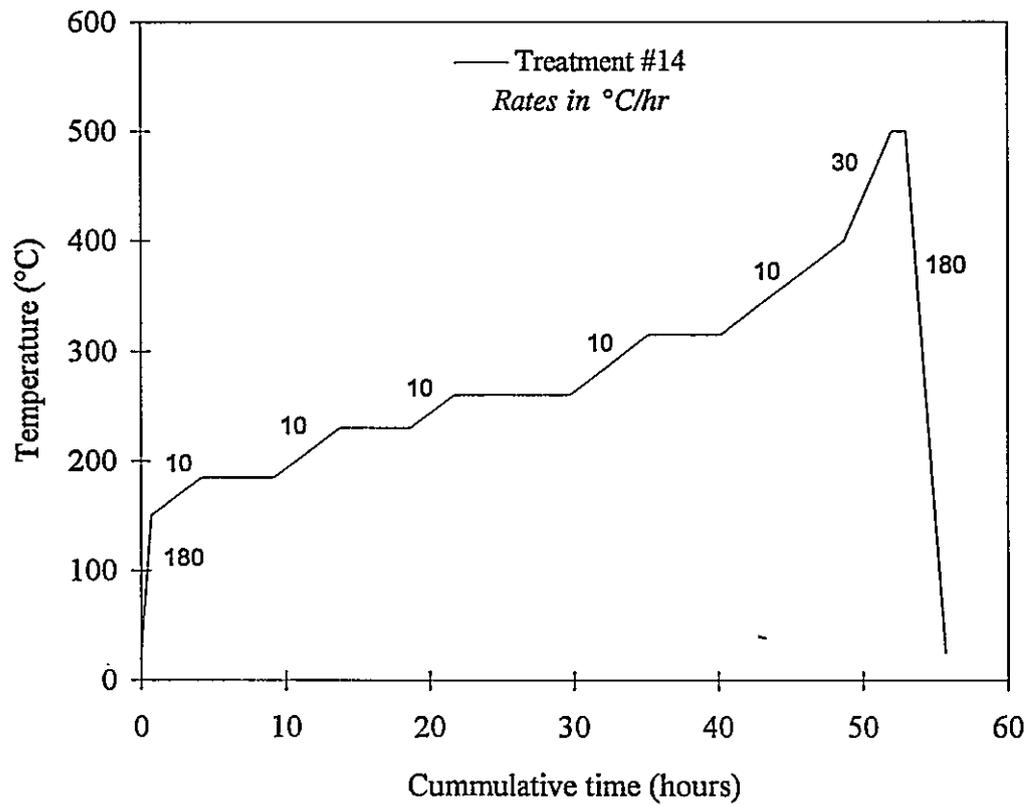
**Figure 3.7:** Burnout treatment of large geometry, nickel laminates in air.
