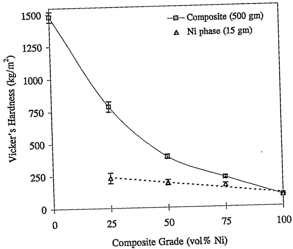
Figure 5.24: Evaluation of composite macrohardness (using 500g load) and nickel phase microhardness (using 15g load) as a function of composite grade.
