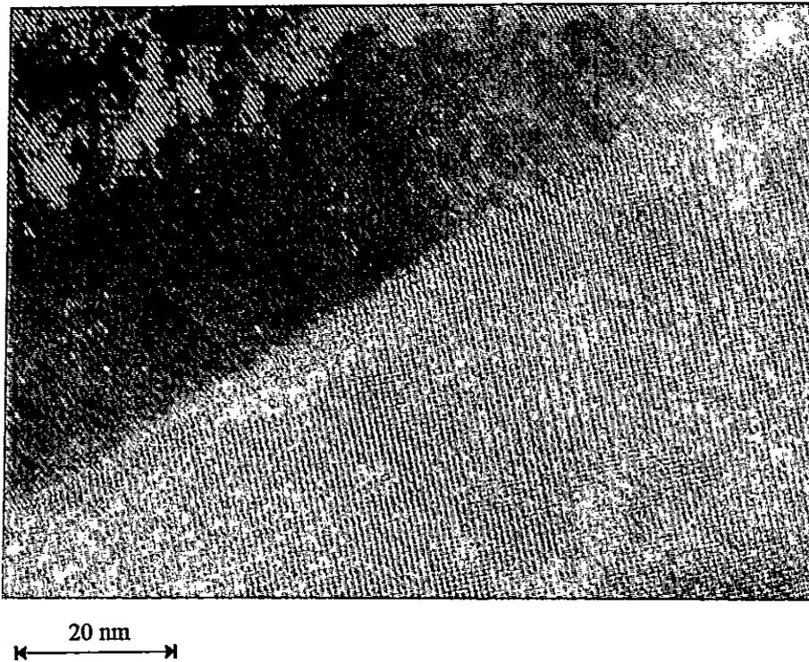
**Figure 5.11:** TEM image of  $ZrO_2$ - $Y_2O_3$  interface in ceramic phase of 50%Ni:50%TZ8Y composite.
