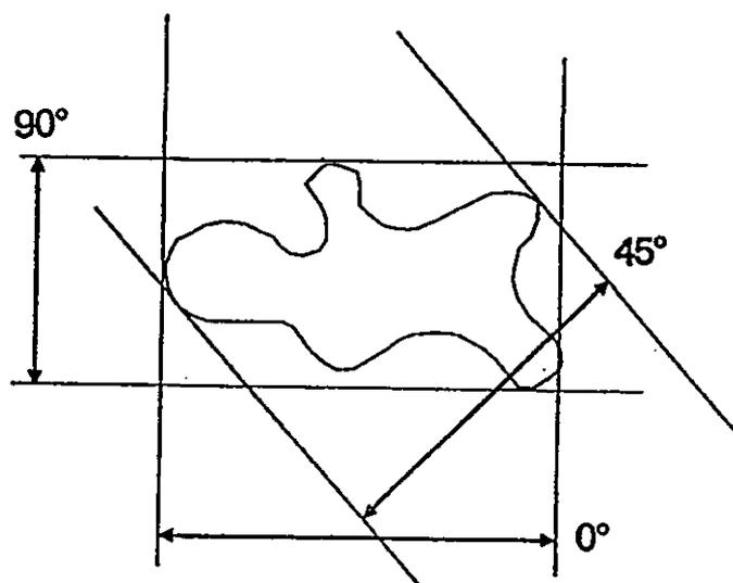
**Figure 5.6:** Schematic representation of ferets (i.e. straight line measurements made between tangents at various angles) shown in three feret angles. (From Leco<sup>®</sup> 2001 reference manual).
