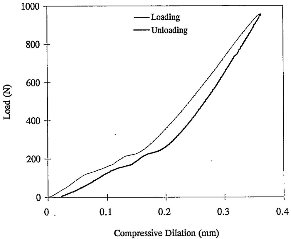
Figure 4.2: System compliance of the Lloyd's materials testing system.
