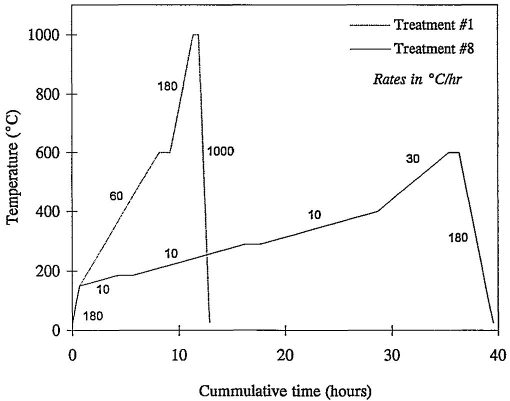
Figure 3.5: Laminate burnout treatments in flowing argon gas.
