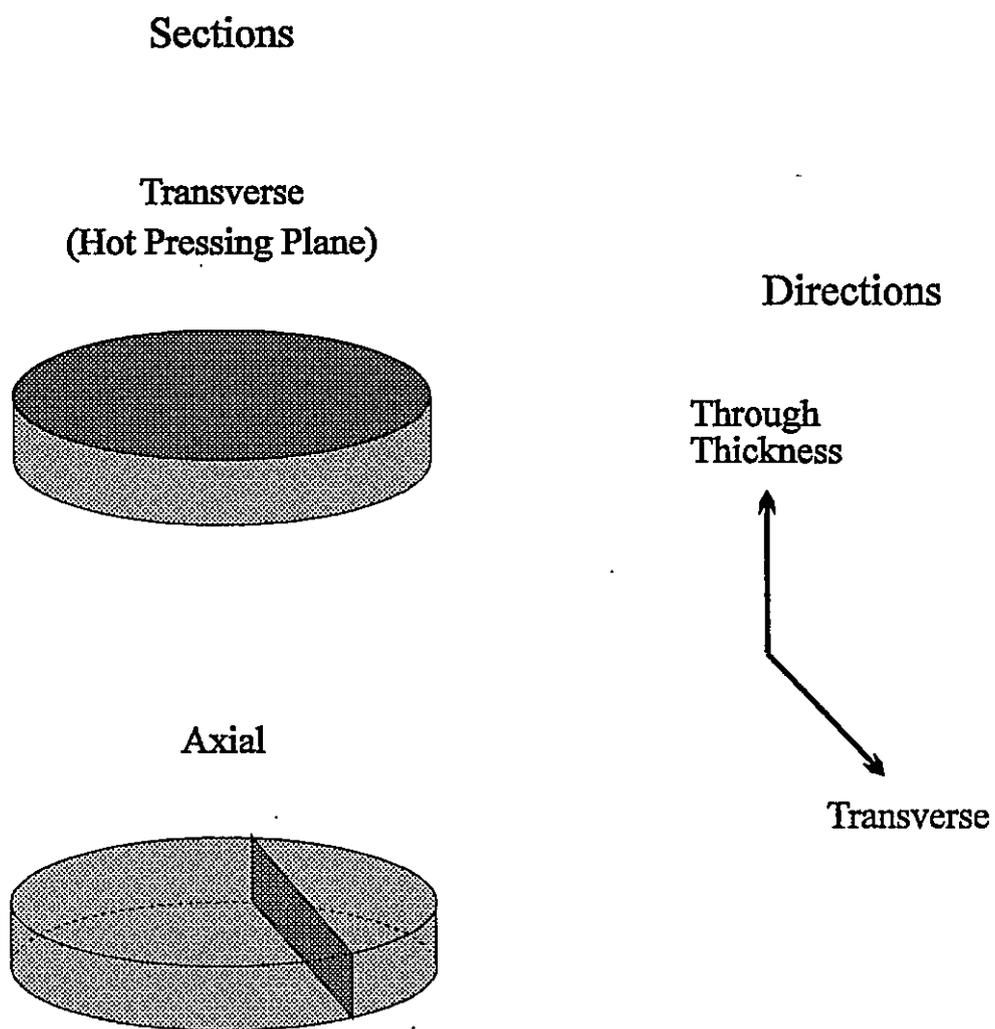
**Figure 5.5:** Schematic of section and direction nomenclature used to characterize composite micrographs.
