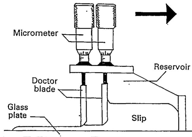
Figure 2.4: (a) Ceramic processing flowsheet (Roosen, 1988), (b) doctor blade apparatus.
