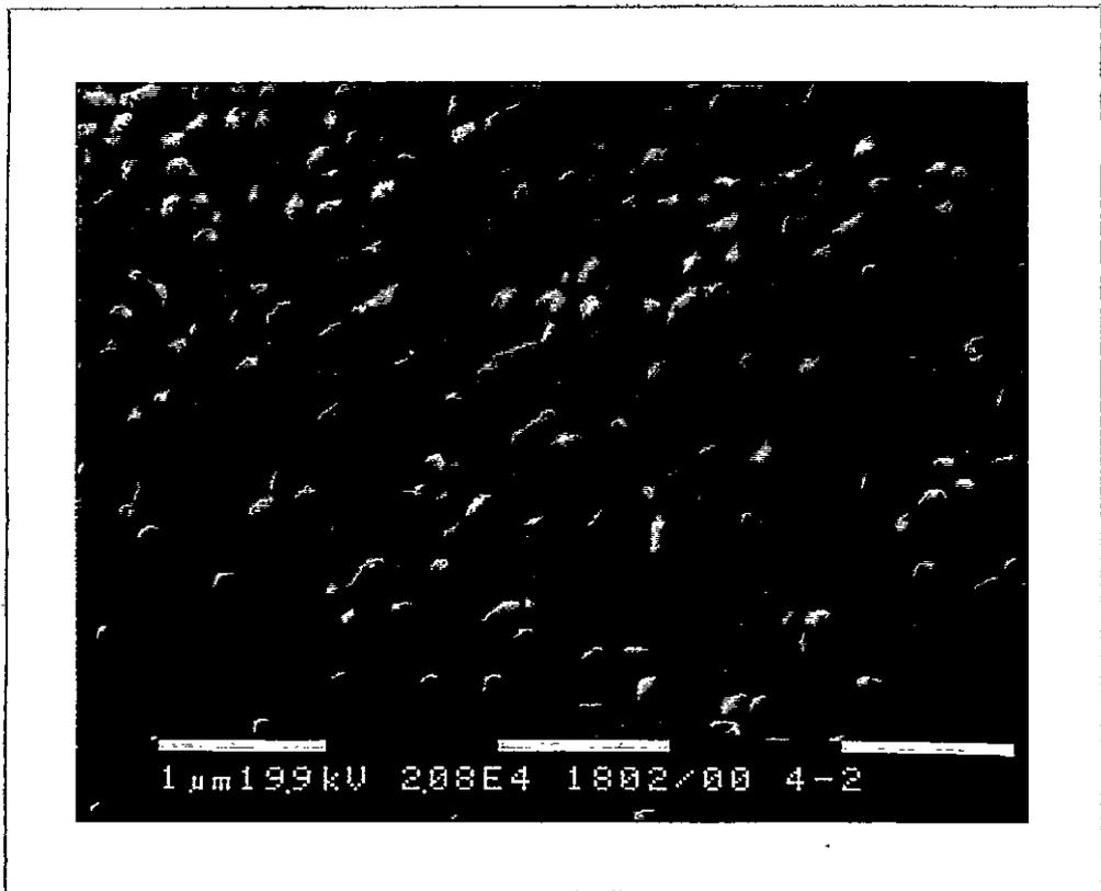
**Figure 5.7:** Grain structure developed in TZ8Y (consolidated at 1250°C for 3 hours and thermally etched at 1200°C for 5 minutes).
