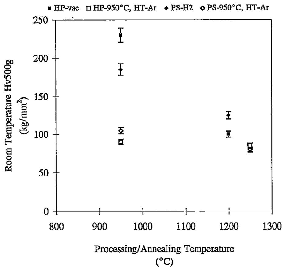
Figure 5.23: The effects of processing and subsequent heat treatment on the hardness of ONF-nickel.
