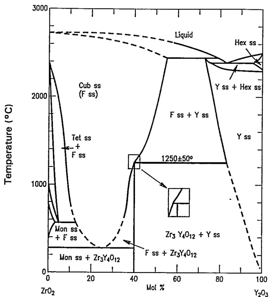
**Figure 6.1:**  $ZrO_2$ - $Y_2O_3$  phase diagram. F = fluorite type of  $ZrO_2$ ; Y =  $Y_2O_3$ ; Cub = cubic; Tet = tetragonal; Mon = monoclinic; Hex = hexagonal. (From Roth, Dennis and McMurdie, 1987).
