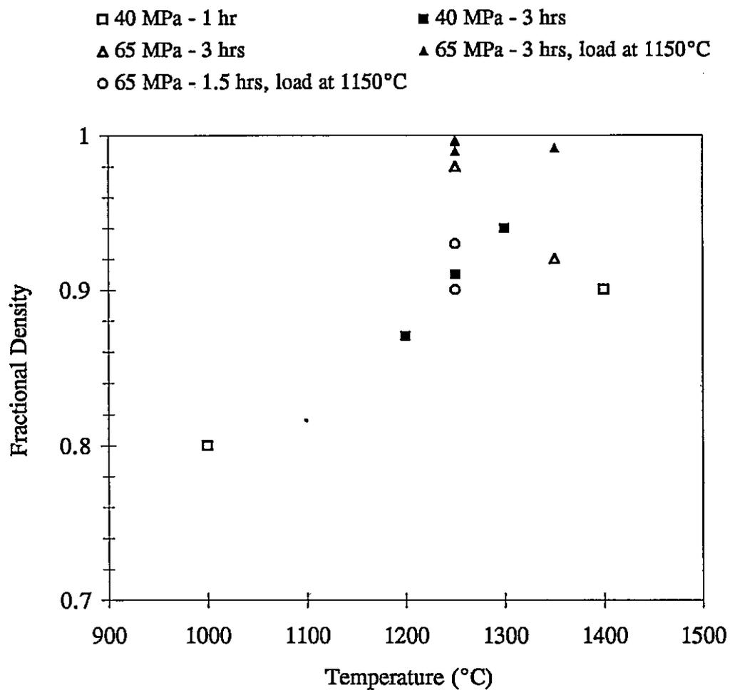
**Figure 3.9:** Effect of hot pressing parameters on the consolidated density of TZ8Y laminates.
