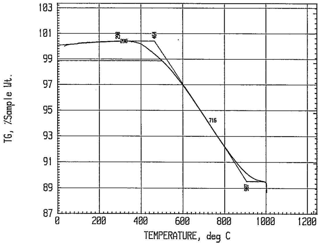
**Figure 3.8:** Reduction of oxidized nickel laminates via thermal treatment in Ar-5% $H_2$  gas. Heating rate of 10°C/minute.
