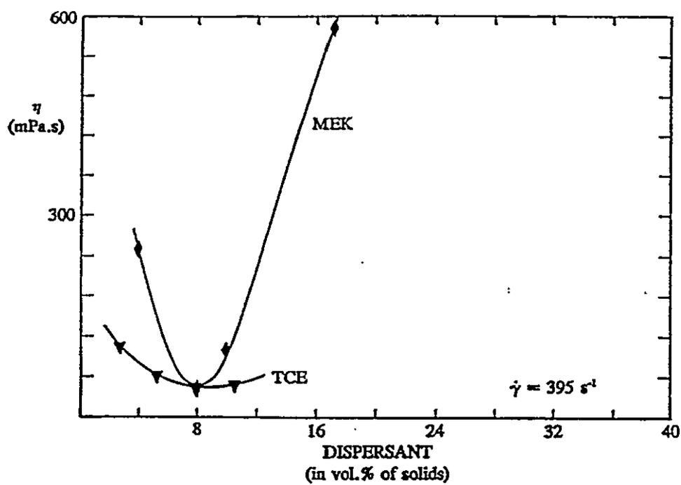
**Figure 2.3:** Effect of phosphate ester-dispersant on alumina slurry viscosity for two different solvents (Plucknett et al., 1994).
