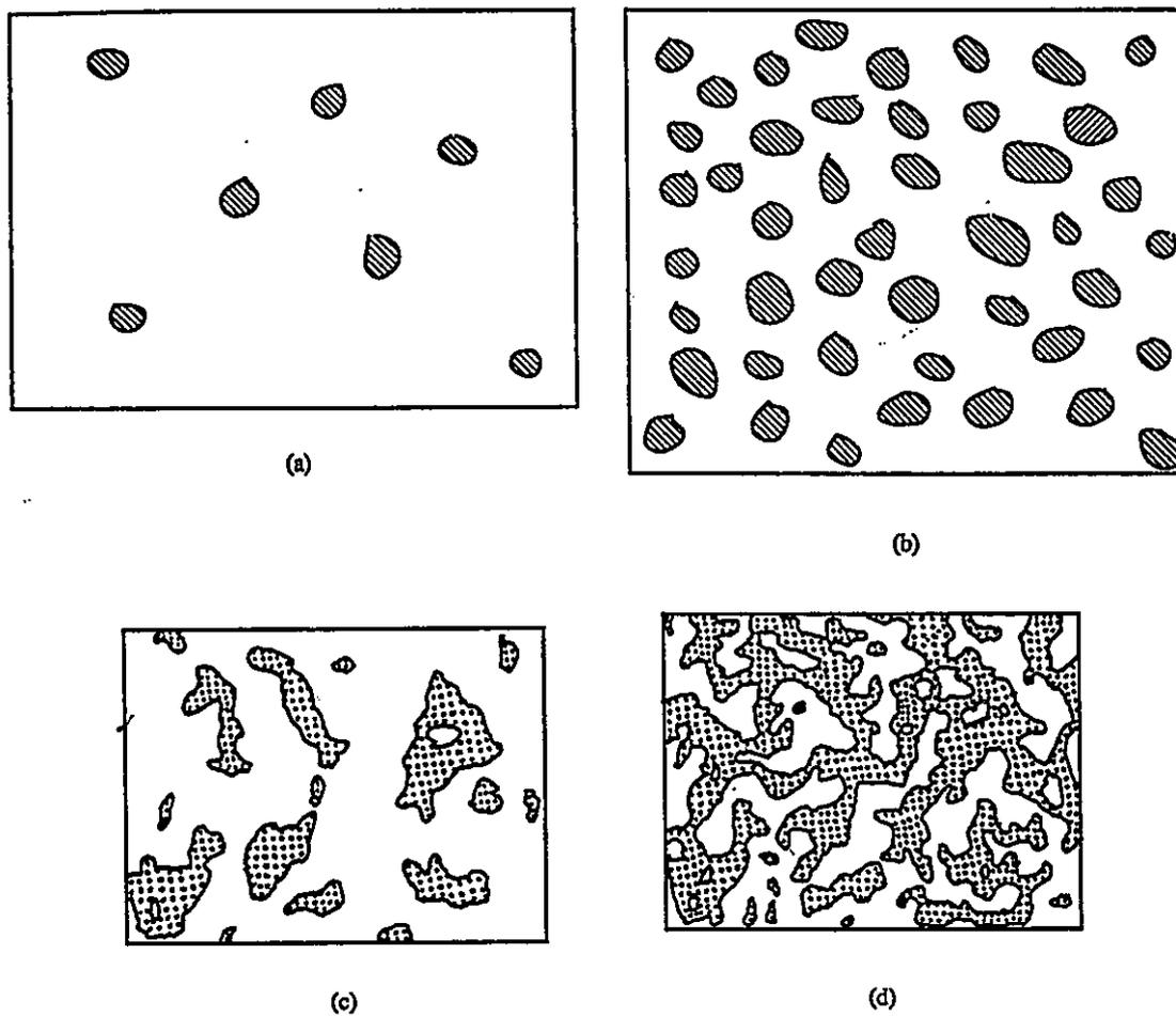
**Figure 2.2:** Schematic microstructure of two-phase heterogeneous materials (Nan, 1993). (a) randomly dispersed grain structure, (b) uniformly dispersed grain structure, (c) aggregated grain structure, (d) percolation-like cluster structure.
