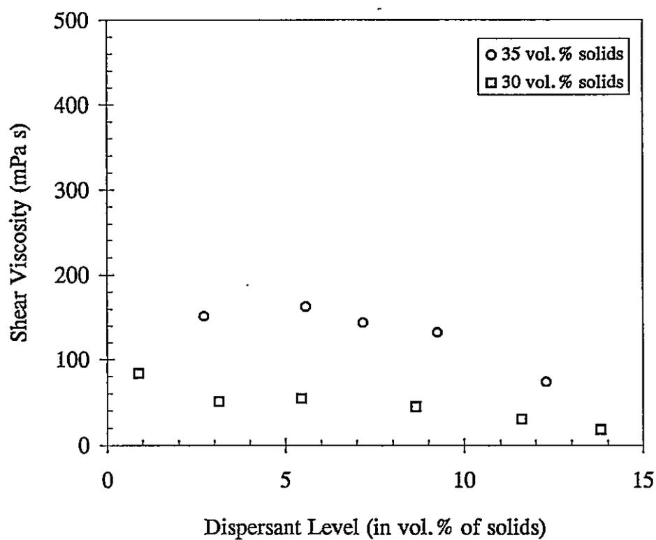
**Figure 3.2:** The shear viscosity-dispersant dependence obtained for slurries containing zirconia powder (TZO), phosphate ester and trichloroethylene.
