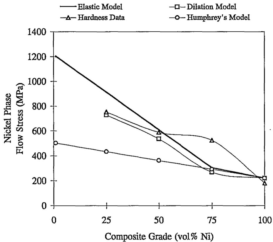
Figure 6.3: Comparison of various models to predict nickel phase flow stress within Ni:TZ8Y composites.
