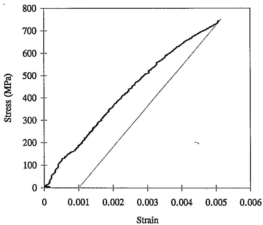
**Figure 5.21:** Tensile profile for ONF-nickel hot pressed at 950°C in vacuum. 0.1% offset yield point indicated.
