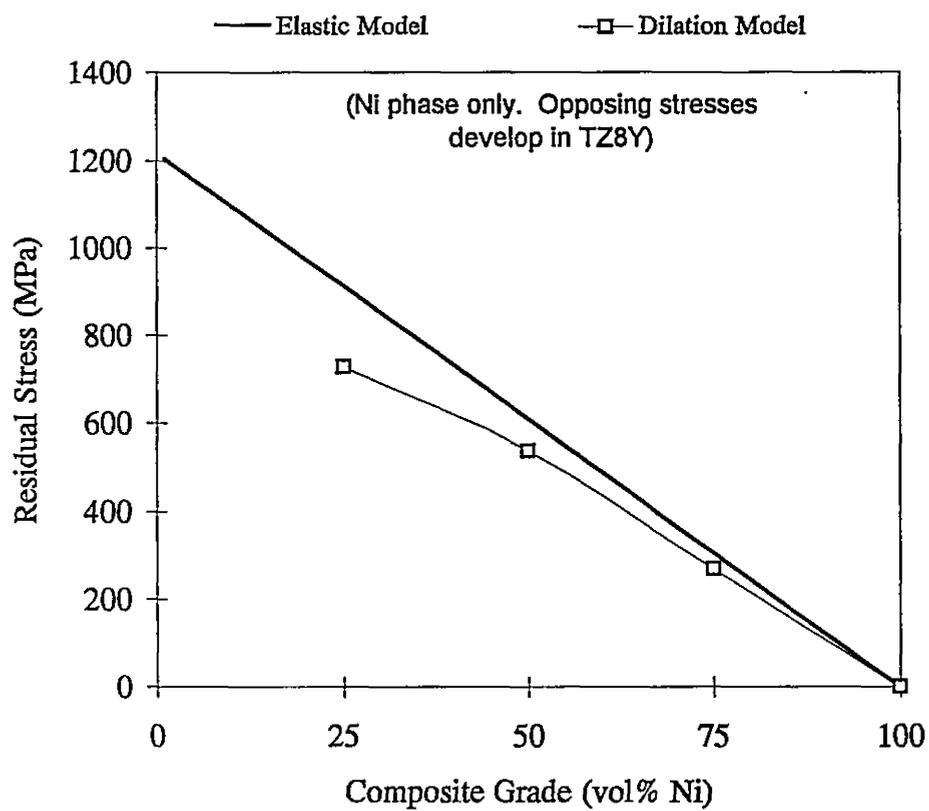
**Figure 6.2:** Residual stress dependence in Ni: TZ8Y composites calculated via continuum mechanics.
