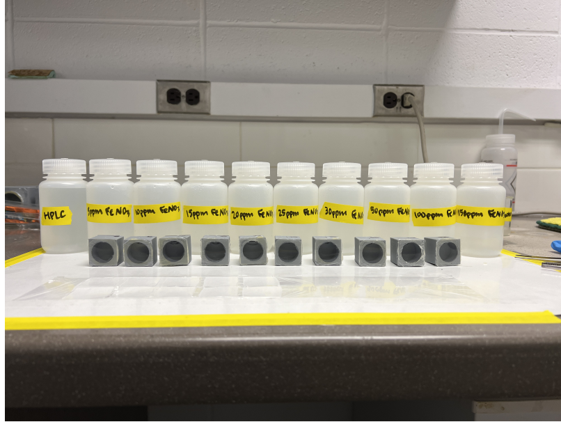
Figure 2.2: Calibration phantoms (grey) with the jars containing iron-doped water solutions behind.
